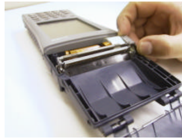
Figure 2.5.4.2 Attaching the printer unit (1/2)
