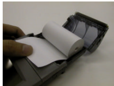
Figure 2.5.3.2 Replacing the roll paper
