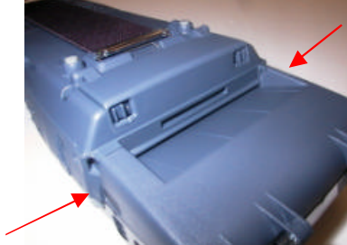
Figure 2.9 Inserting and removing memory cards (1/4)
