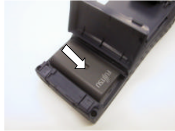
Figure 2.6.2 Replacing the lithium-ion battery pack (3/3)
