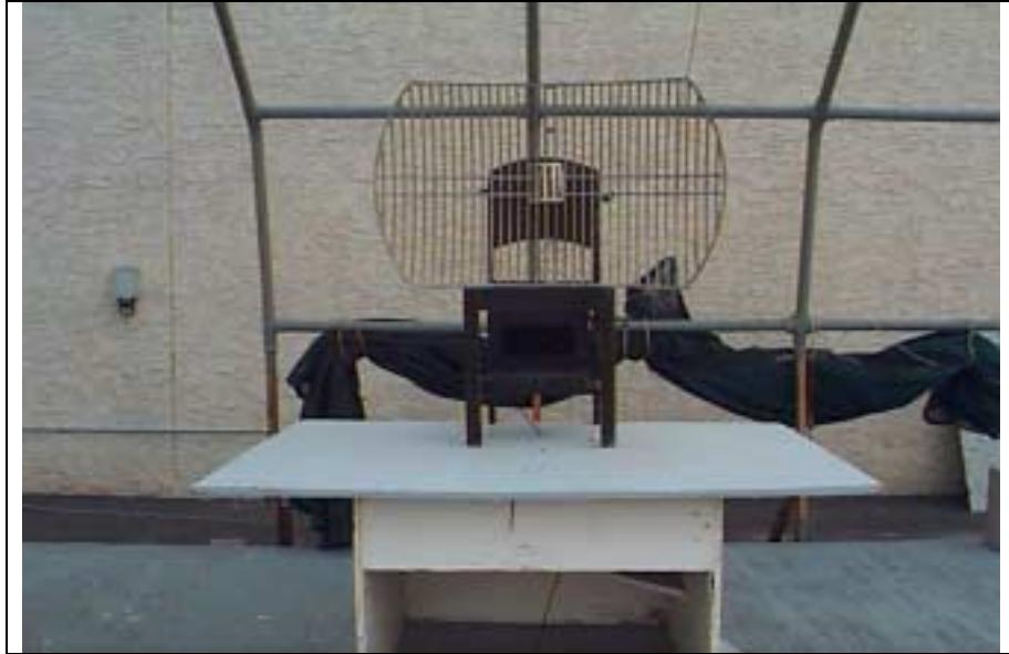
TEST SETUP: Radiated Emissions
