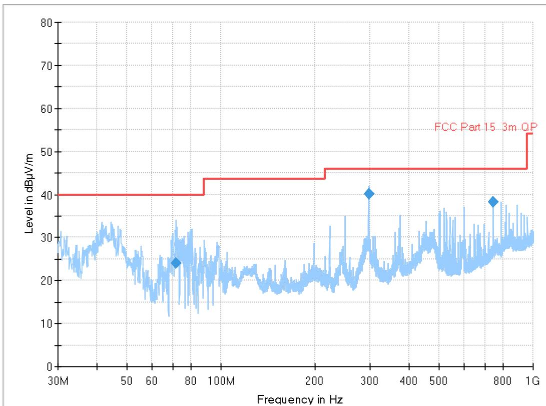
Radiated Emissions 30 - 1000 MHz, GFSK
