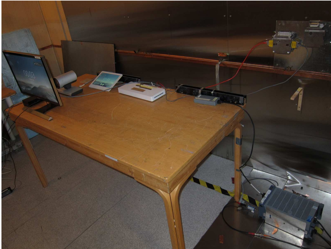
Power line Conducted Emissions Test
