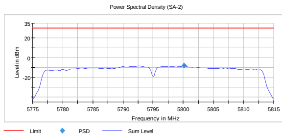
PSD, 5795 MHz, 802.11ac, HT40, MCS0, MIMO -8.2 dBm
