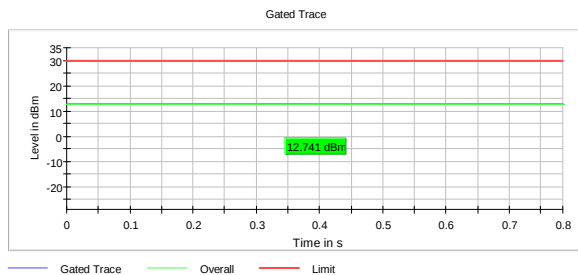
RMS Conducted Power, 5755 MHz, 802.11ac, HT40, MCS0, MIMO
