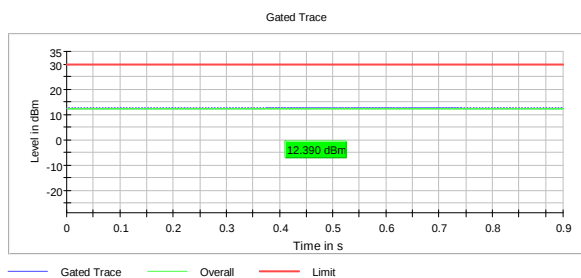
RMS Conducted Power, 5825 MHz, 802.11a, 6Mb
