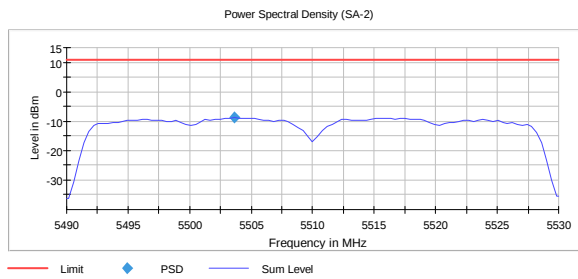
PSD, 5510 MHz, 802.11ac, HT40, MCS8 -8.9 dBm
