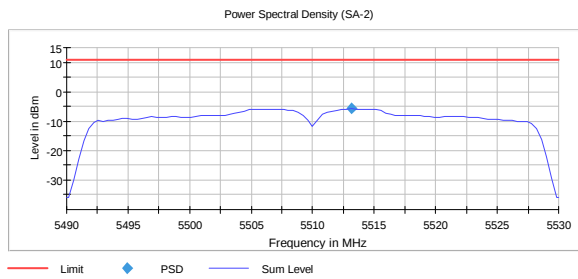
PSD, 5510 MHz, 802.11ac, HT40, MCS0, MIMO -5.8 dBm
