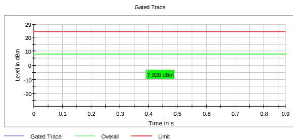
RMS Conducted Power, 5320 MHz, 802.11n, HT20, MCS8, MIMO
