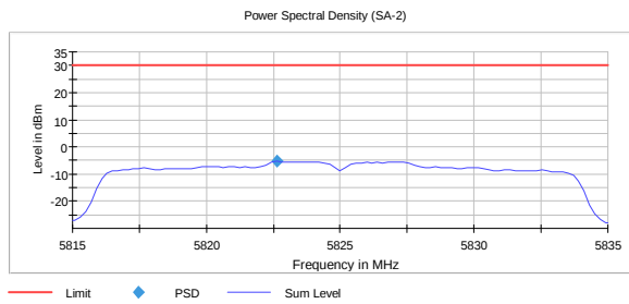
PSD, 5825 MHz, 802.11n, HT20, MCS8, MIMO -5.4 dBm
