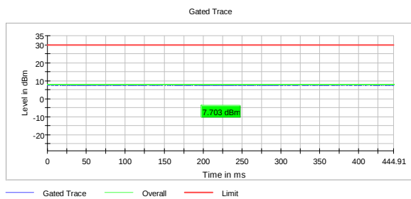
RMS Conducted Power, 5775 MHz, 802.11ax, HT80, MCS11, MIMO
