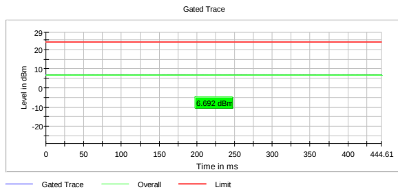
RMS Conducted Power, 5210 MHz, 802.11ax, HT80, MCS11, MIMO
