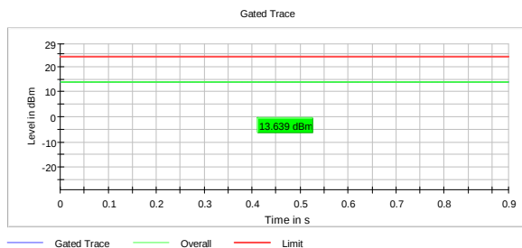
RMS Conducted Power, 5240 MHz, 802.11a, 6Mb
