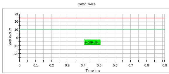
RMS Conducted Power, 5280 MHz, 802.11ax, HT20, MCS0, MIMO
