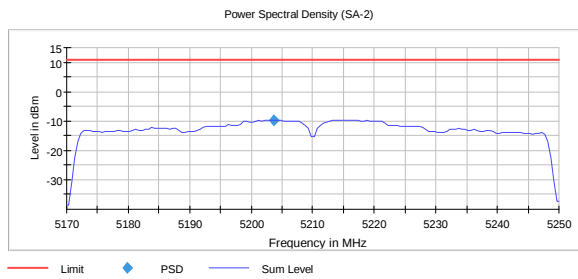
PSD, 5210 MHz, 802.11ac, HT80, MCS0 -9.7 dBm
