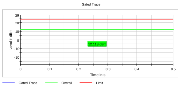
RMS Conducted Power, 5720 MHz, 802.11ax, HT20, MCS0, MIMO
