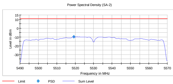
PSD, 5530 MHz, 802.11ac, HT80, MCS0 -9.8 dBm
