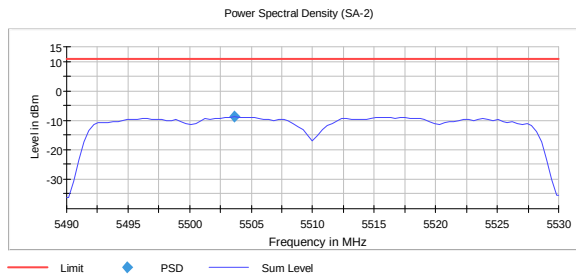
PSD, 5510 MHz, 802.11ac, HT40, MCS8 -8.9 dBm
