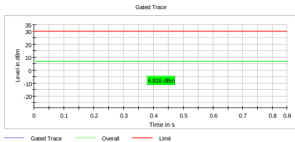
RMS Conducted Power, 5795 MHz, 802.11ax, HT40, MCS0, MIMO
