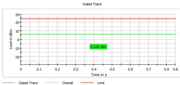
RMS Conducted Power, 5190 MHz, 802.11ax, HT40, MCS0, MIMO
