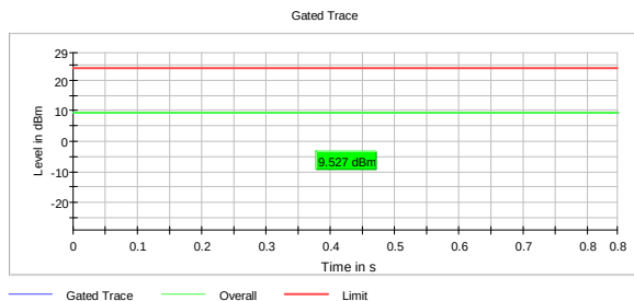
RMS Conducted Power, 5270 MHz, 802.11ax, HT40, MCS0, MIMO
