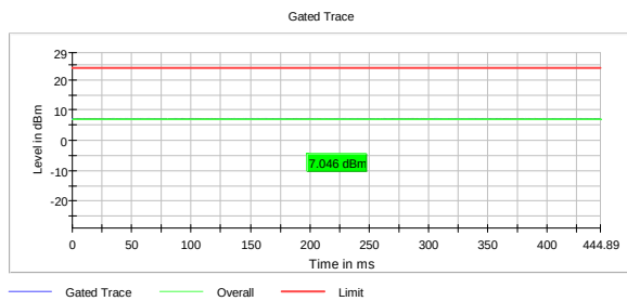
RMS Conducted Power, 5530 MHz, 802.11ax, HT80, MCS11, MIMO
