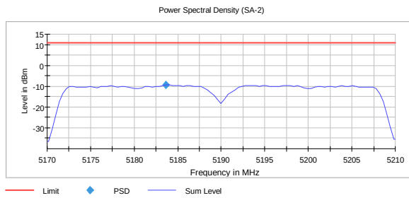
PSD, 5190 MHz, 802.11ac, HT40, MCS8 -9.4 dBm
