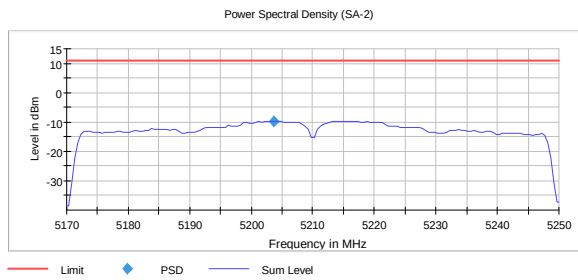
PSD, 5210 MHz, 802.11ac, HT80, MCS0 -9.7 dBm
