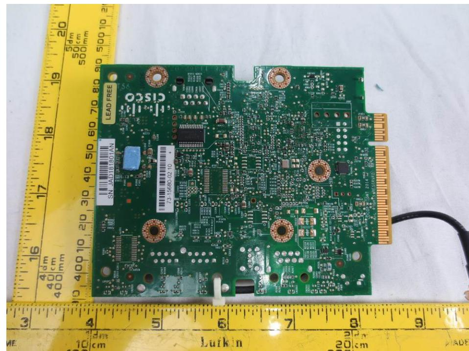
**17.37 Advance Range Extender Interface Board, Top View**
