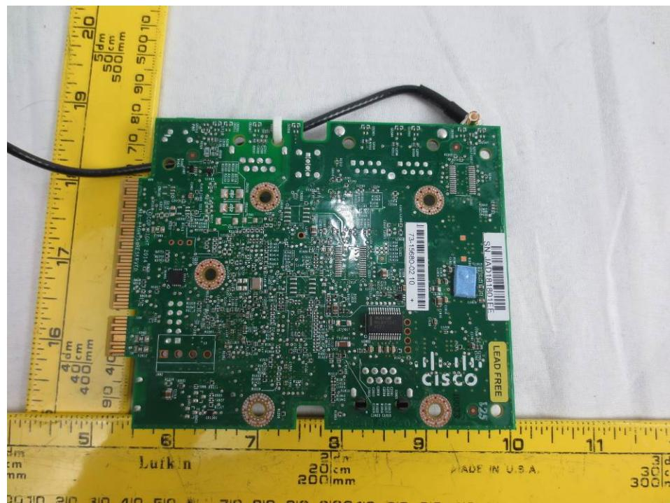
**17.25 Advance Range Extender Interface Board, Top View**
