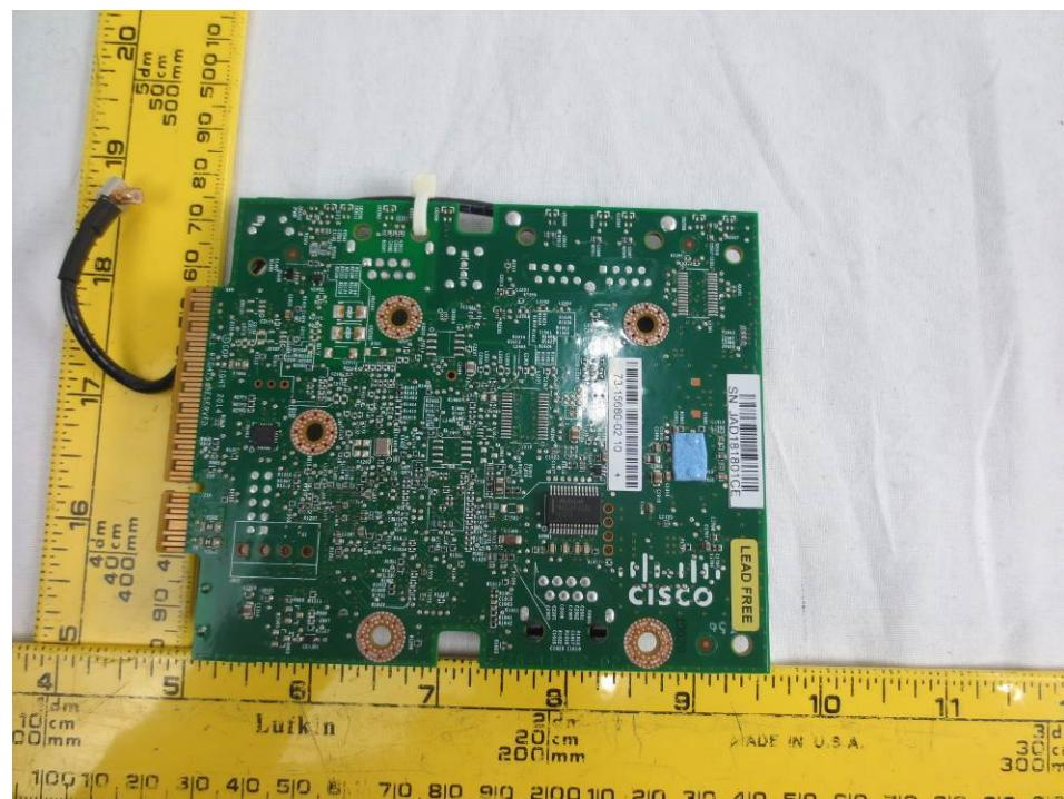
**Model: IR529UBWP-915S/K9****17.21 Power Board, Top View**
