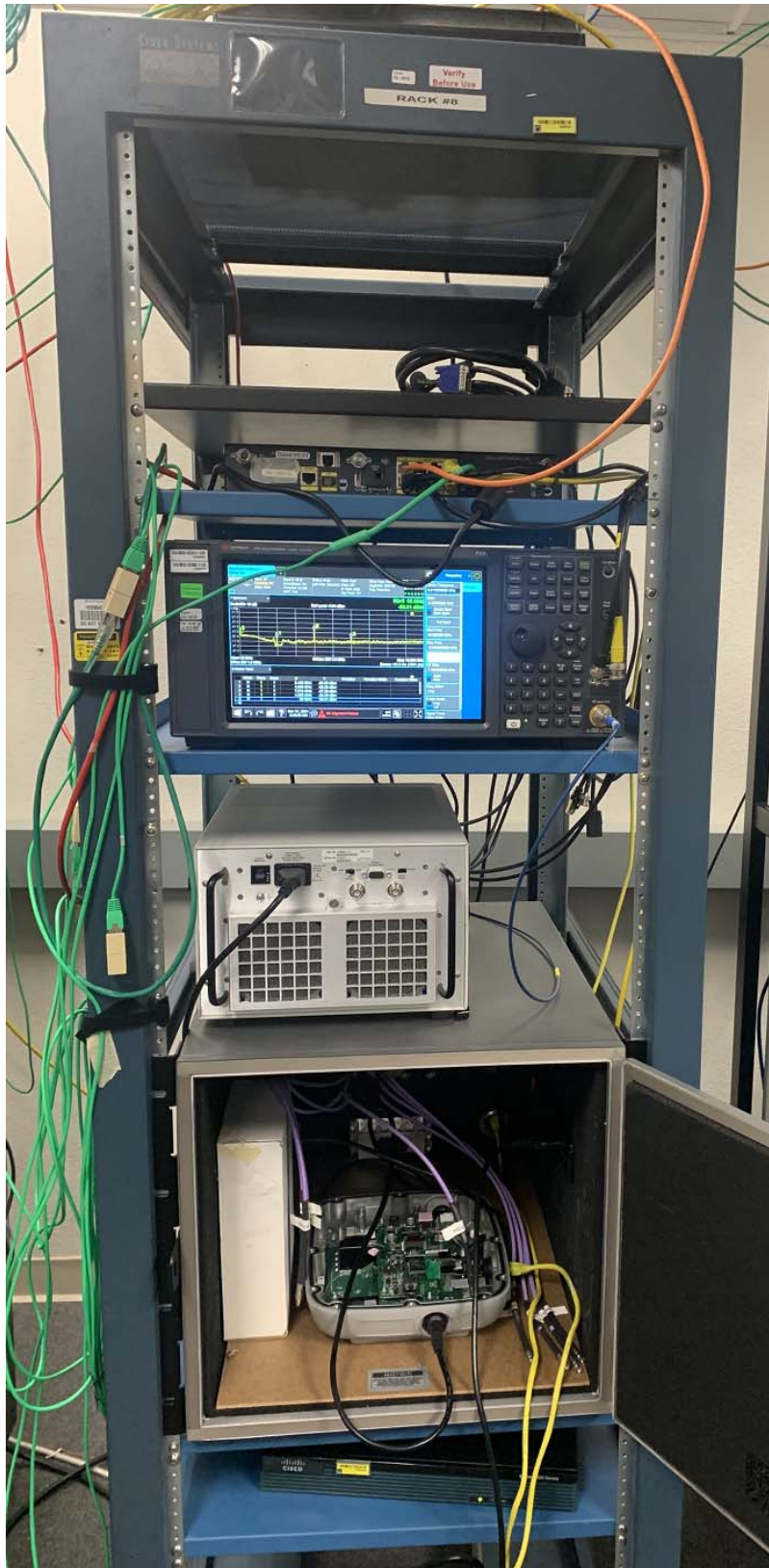
Title: Radio Conducted Test Setup – Rack 8 - BLE
