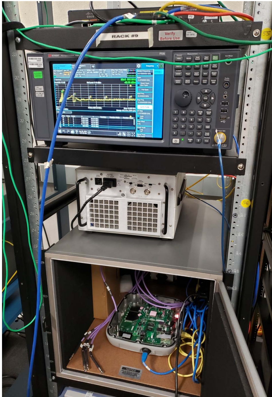
Title: Radio Conducted Test Setup – Rack 9
