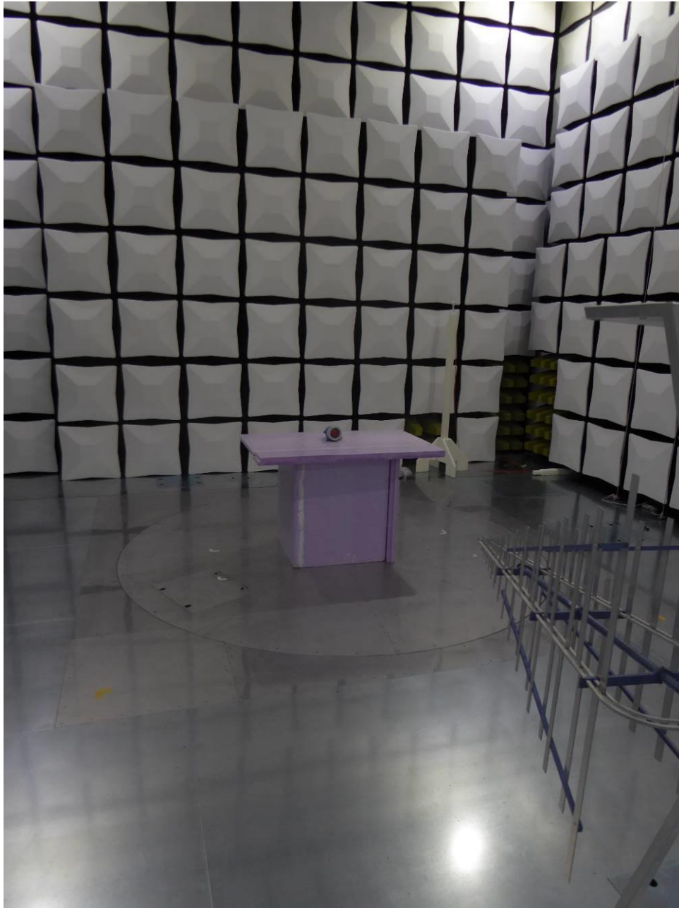
Test setup – radiated test in anechoic chamber (M276)
