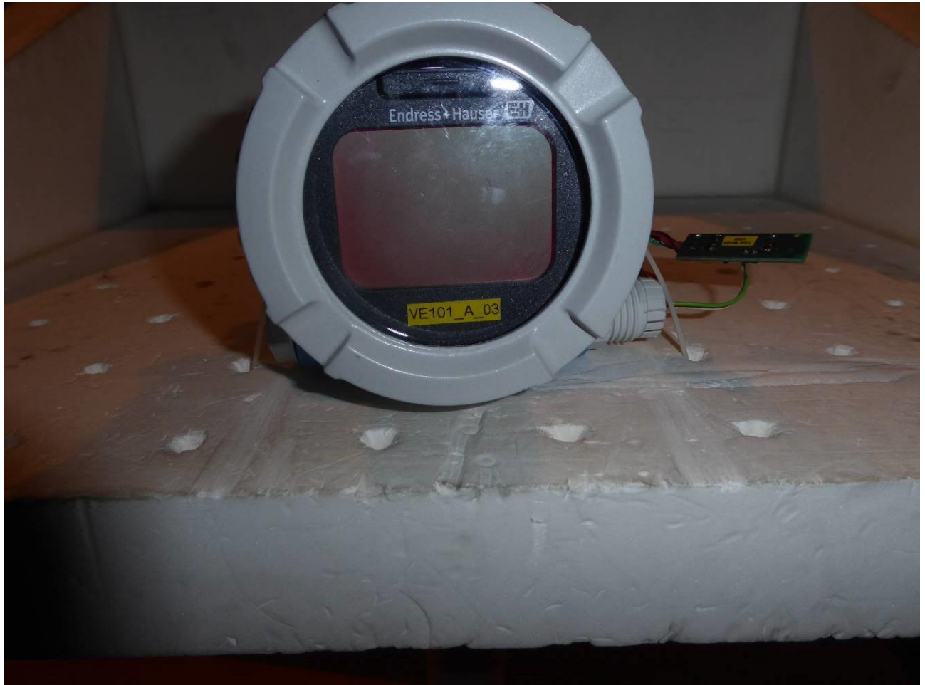
Test setup – radiated test in anechoic chamber
