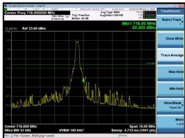
LTE Band 12 QPSK 3MHz CH-High, 1 RB
