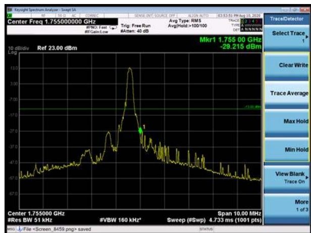
LTE Band 4 16QAM 3MHz CH-High, 1 RB
