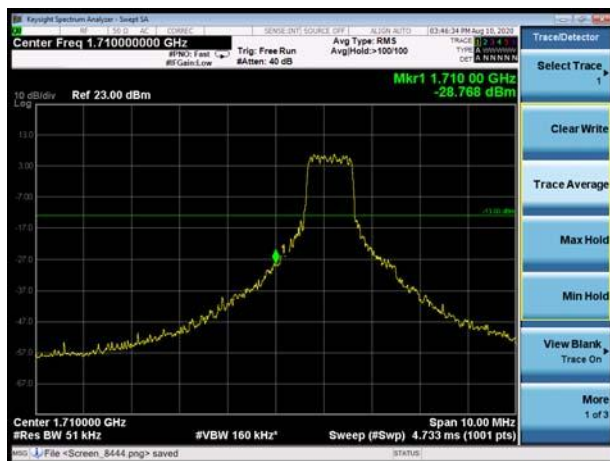
LTE Band 4 16QAM 15MHz CH-Low, 1 RB
