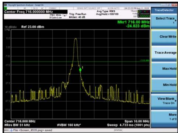
LTE Band 12 16QAM 5MHz CH-High, 100%RB
