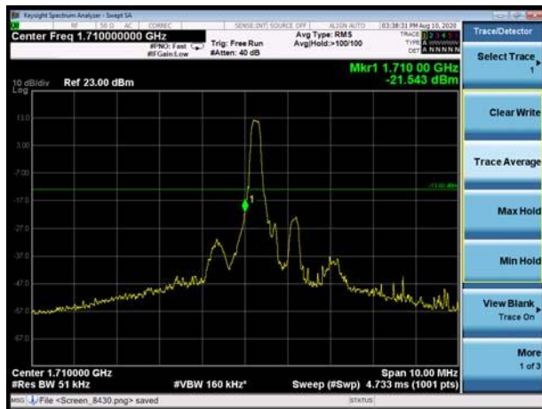
LTE Band 4 16QAM 1.4MHz CH-Low, 100%RB
