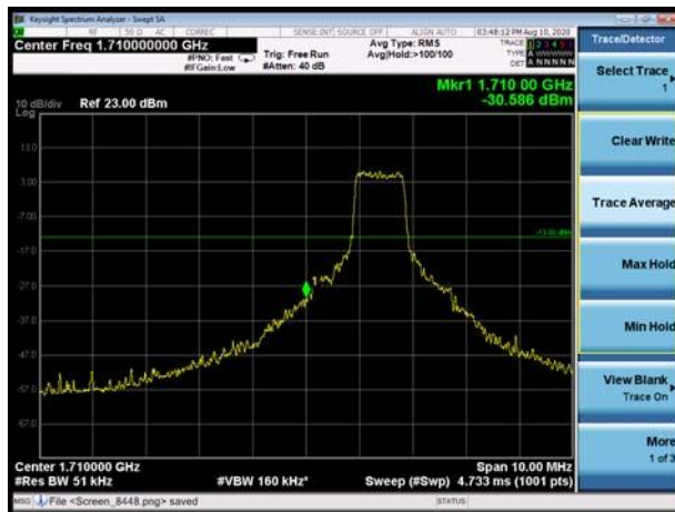
LTE Band 4 16QAM 20MHz CH-Low, 1 RB
