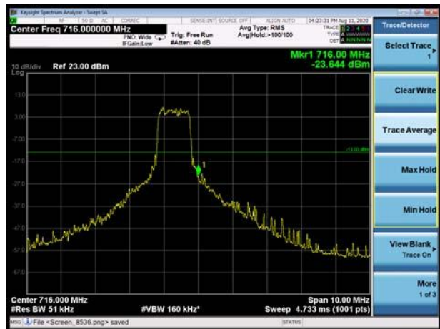
LTE Band 12 16QAM 10MHz CH-High, 1 RB
