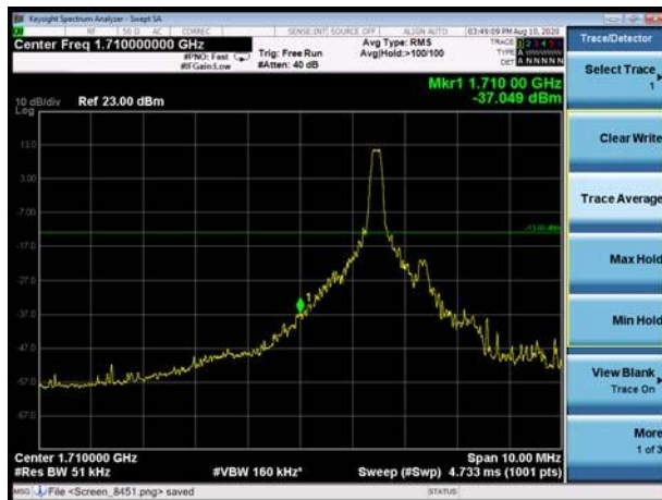
LTE Band 4 16QAM 20MHz CH-Low, 100%RB
