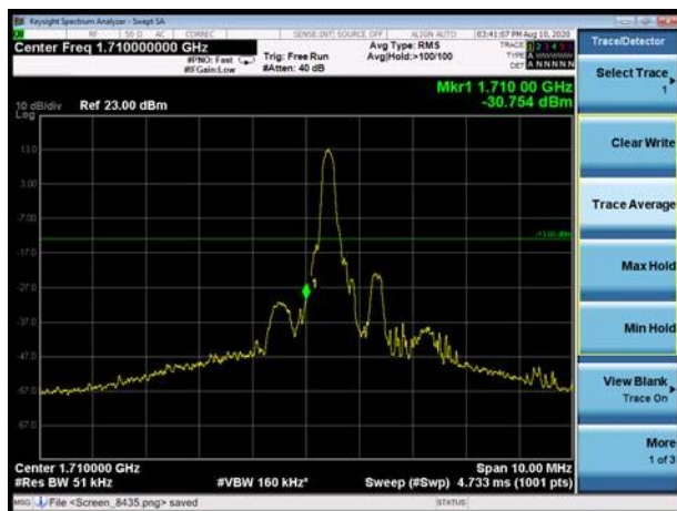
LTE Band 4 16QAM 3MHz CH-Low, 1 RB
