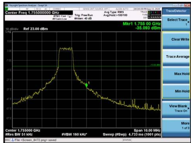
LTE Band 4 16QAM 20MHz CH-High, 1 RB
