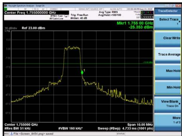
LTE Band 4 QPSK 3MHz CH-High, 1 RB
