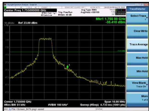
LTE Band 4 QPSK 20MHz CH-High, 100%RB
