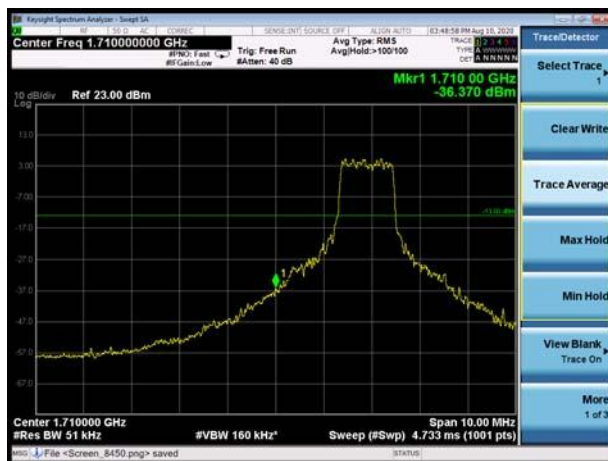
LTE Band 4 QPSK 20MHz CH-Low, 100%RB
