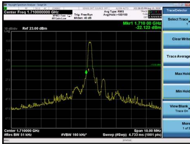
LTE Band 4 QPSK 1.4MHz CH-Low, 100%RB
