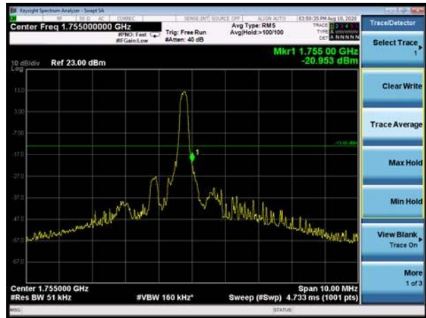
LTE Band 4 QPSK 1.4MHz CH-High, 100%RB
