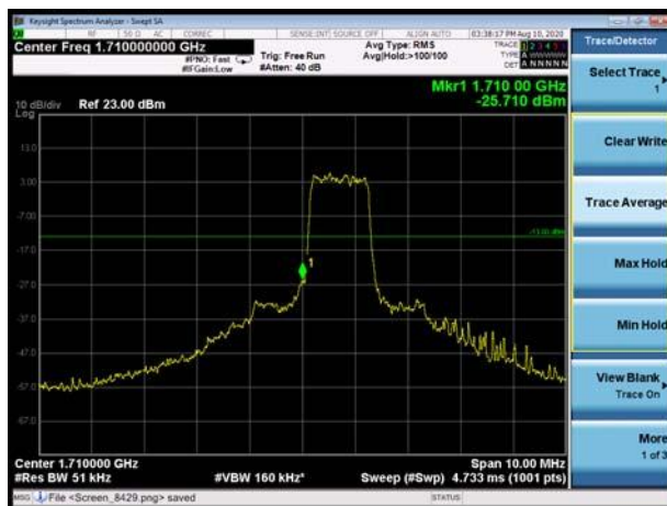
LTE Band 4 QPSK 3MHz CH-Low, 1 RB
