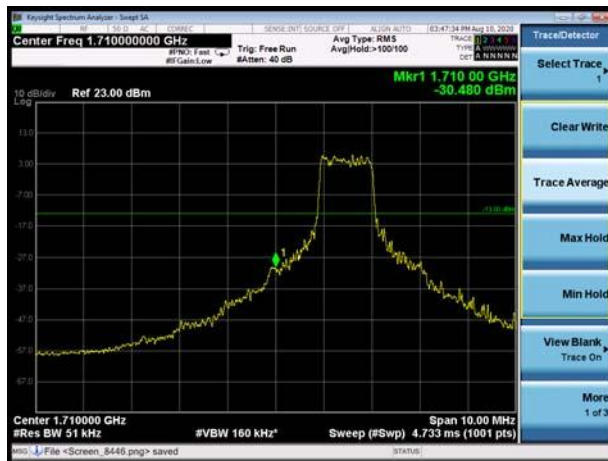
LTE Band 4 QPSK 20MHz CH-Low, 1 RB
