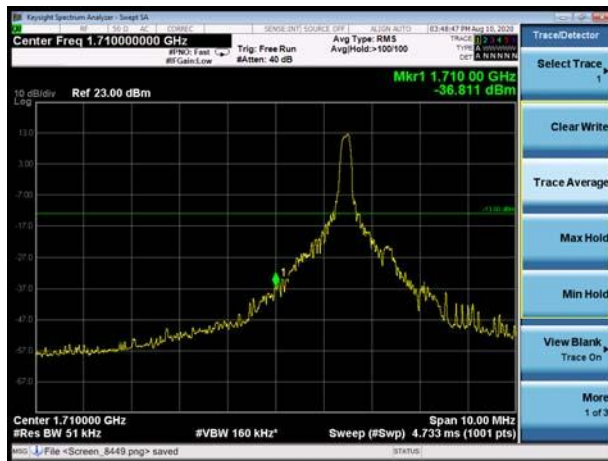
LTE Band 4 QPSK 20MHz CH-Low, 100%RB
