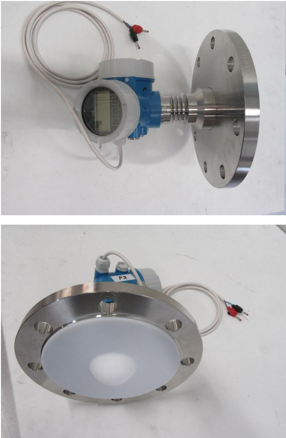
Figure 2 – EUT P3 (FMR51 with antenna Horn 40mm/1-1/2")
