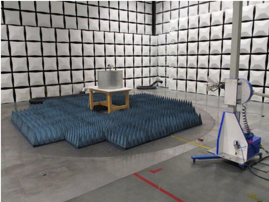
Figure 6 - Test setup for radiated emission on TLPR
