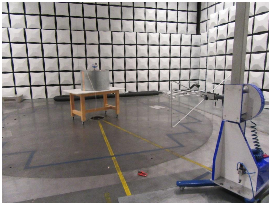
Figure 5 - Test setup for radiated emission on TLPR
