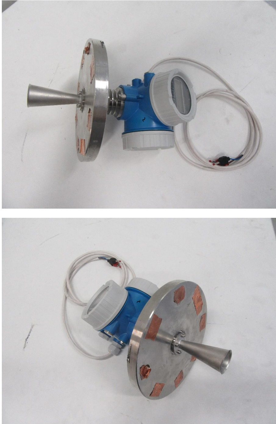
Figure 1 – EUT P2 (FMR50 with antenna Horn 100mm/4" PP cladded
