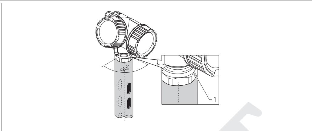
**16 Installation in stilling well****1 Marking for antenna alignment**
