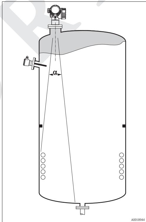
Avoid any installations (limit switches, temperature sensors, braces, vacuum rings, heating coils, baffles etc.) inside the signal beam. Take into account the beam angle (→ 38):
