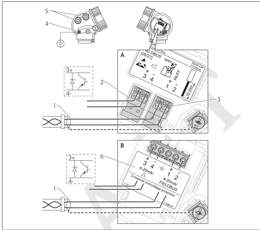
8 Terminal assignment PROFIBUS PA / FOUNDATION Fieldbus
