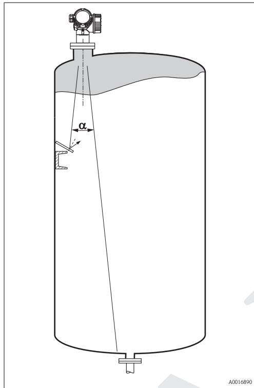
Metallic screens mounted at a slope spread the radar signal and can, therefore, reduce interference echoes.
