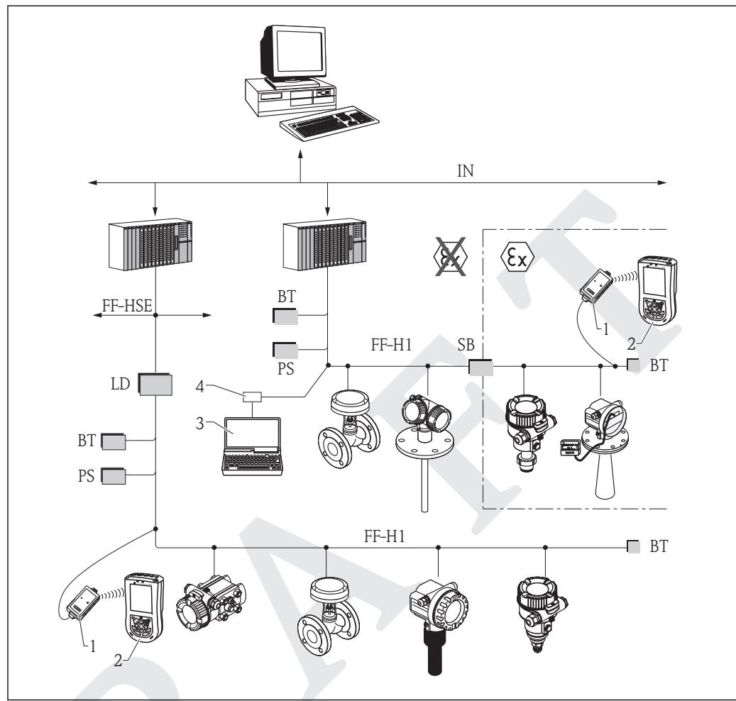
23 FOUNDATION Fieldbus system architecture with associated components
