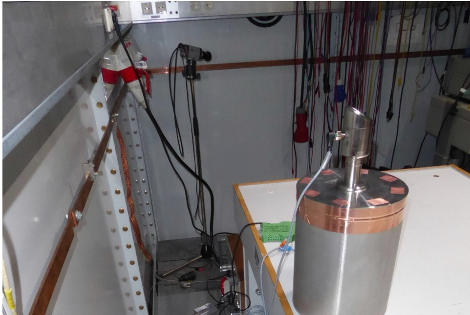
Test setup shielded room M4 Preliminary and final measurement 150 kHz – 30 MHz
