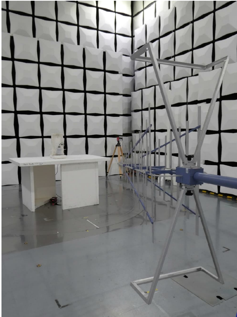
Test setup semi anechoic chamber with EUT 2A (<1 GHz, position 2)
