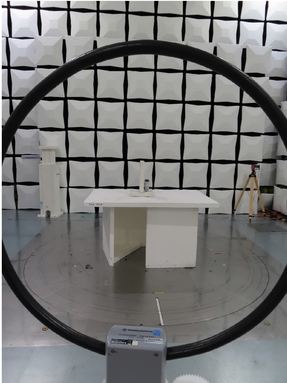
Test setup semi anechoic chamber with EUT 3 (<30 MHz, position 2)
