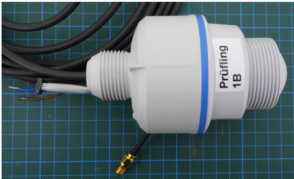
EUT for conducted tests - bottom view
