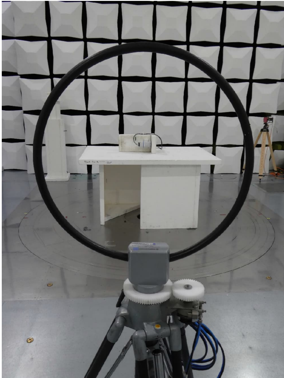
Test setup semi anechoic chamber with EUT 2A (<30 MHz, position 1)
