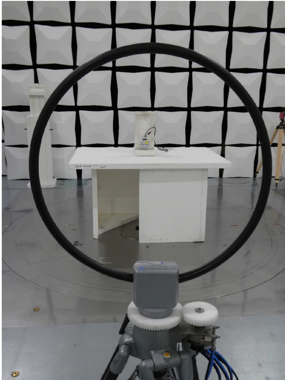
Test setup semi anechoic chamber with EUT 1A (<30 MHz, position 2)
