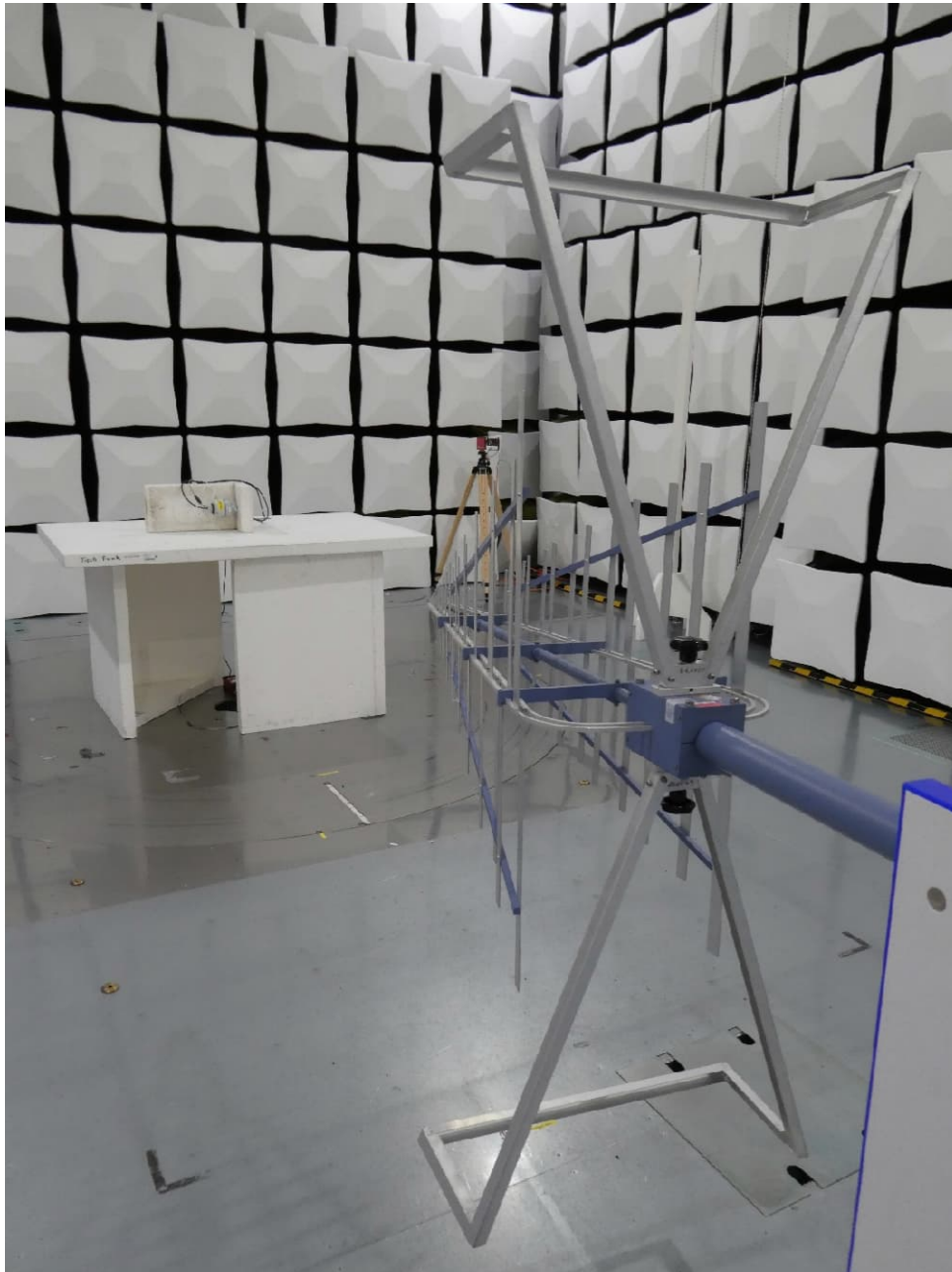
Test setup semi anechoic chamber with EUT 1A (<1 GHz, position 1)
