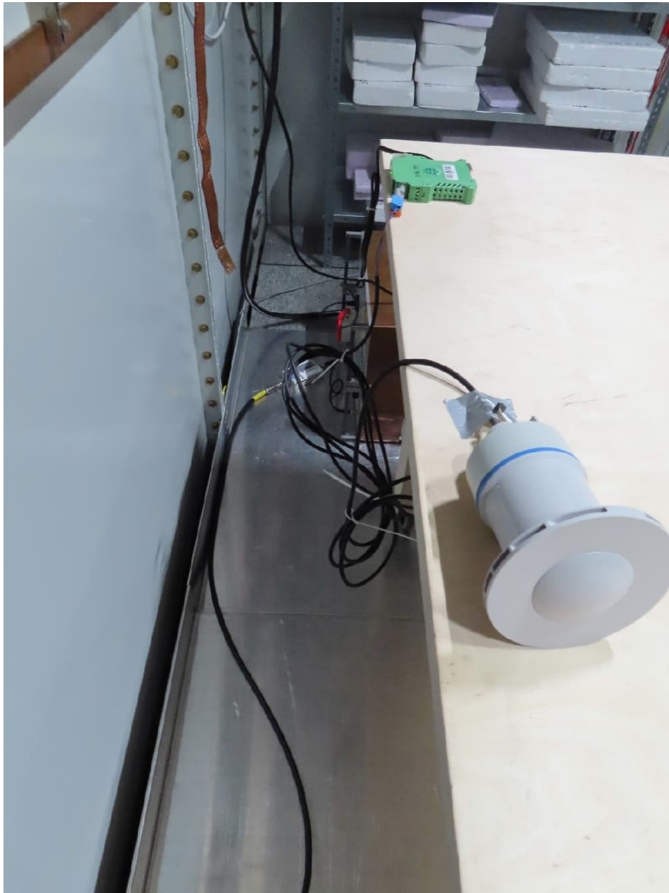
Test AC power line conducted emissions with EUT 2A
