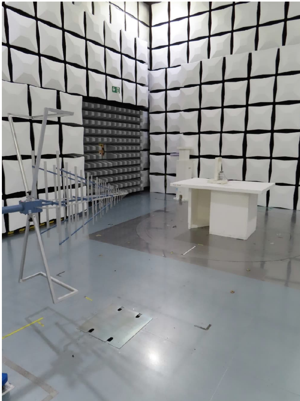
Test setup semi anechoic chamber with EUT 3 (<1 GHz, position 2)
