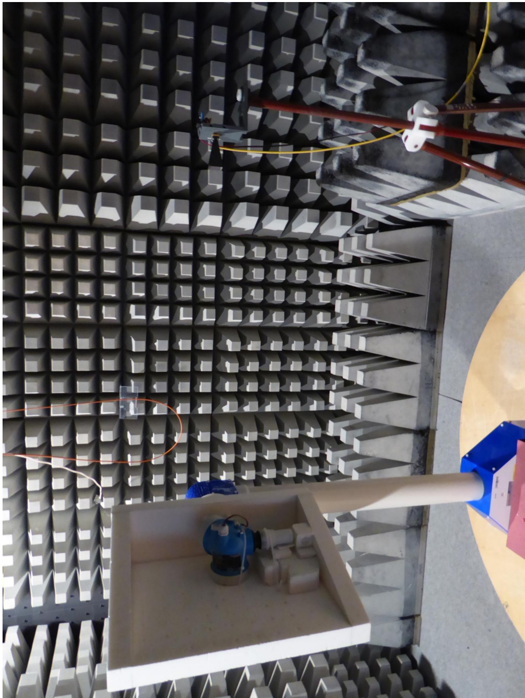
172289_205.JPG: ProToF BTLE-adaptor 2.4 GHz inside FMR50, test setup fully anechoic chamber (26.5 GHz to 40 GHz)
