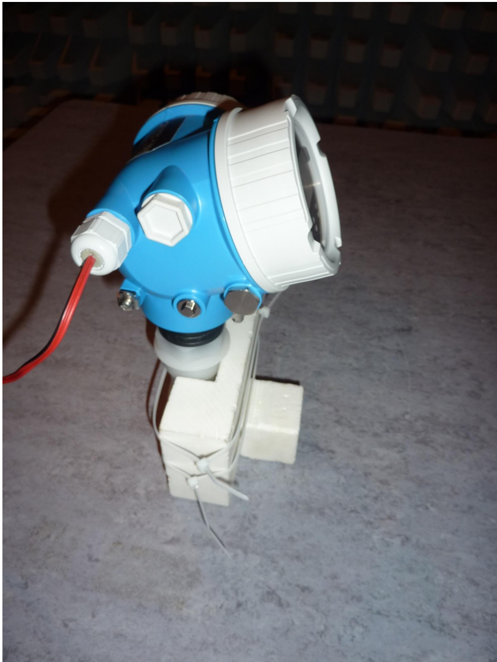
172289_206.JPG: ProToF BTLE-adaptor 2.4 GHz inside FMR50, test setup fully anechoic chamber (pos. 1, 40 GHz to 100 GHz)
