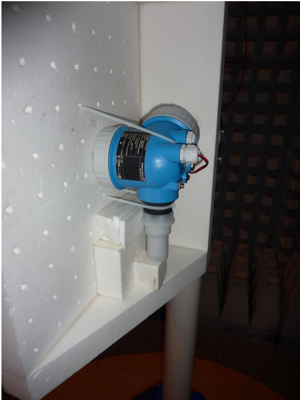
172289_201.JPG: ProToF BTLE-adaptor 2.4 GHz inside FMR50, test setup fully anechoic chamber (pos. 1)
