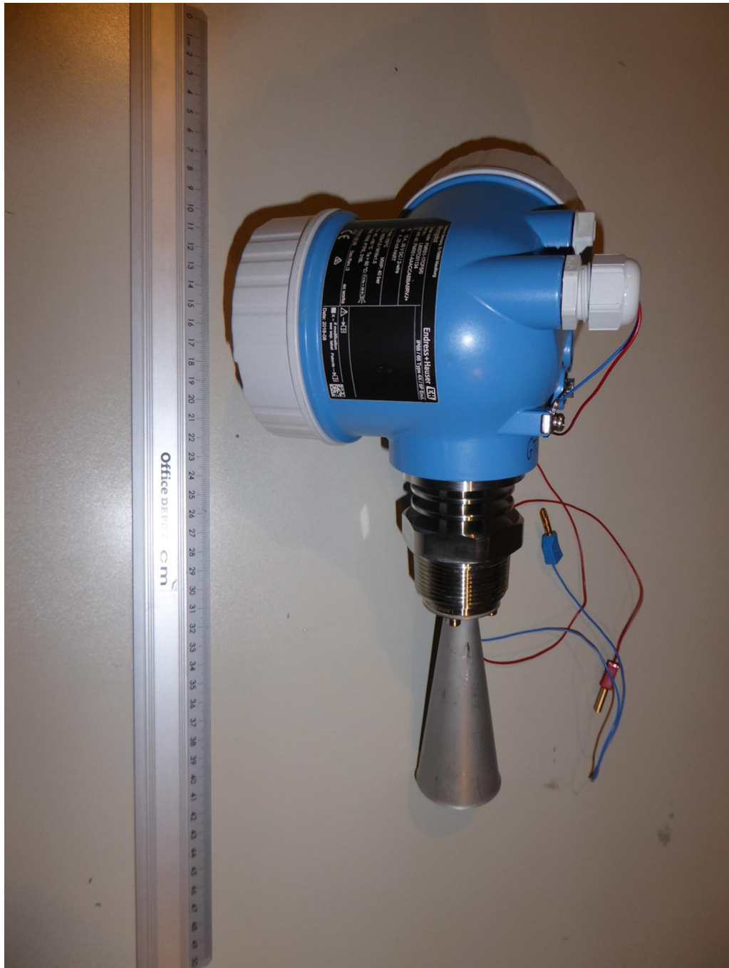
172289_a.JPG: ProToF BTLE-adaptor 2.4 GHz inside FMR51, external view 1
