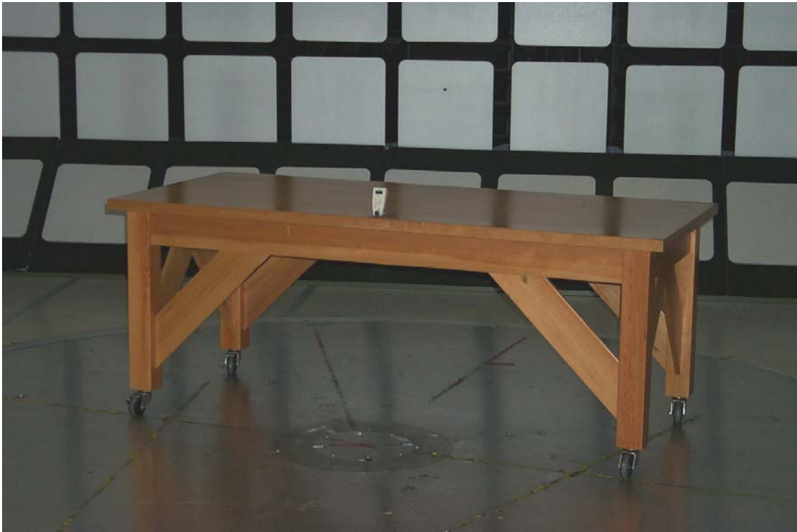
Radiated Emissions Test Setup, EUT Vertical
