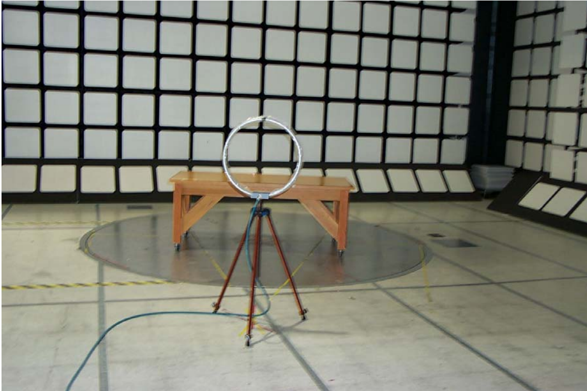
Radiated Emissions Test Setup, 3m distance, Loop Antenna
