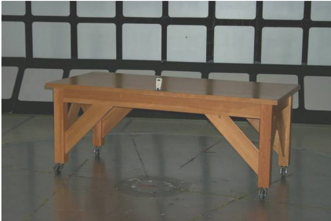
Figure 2 - Radiated Emissions Test Setup, Vertical EUT Position
