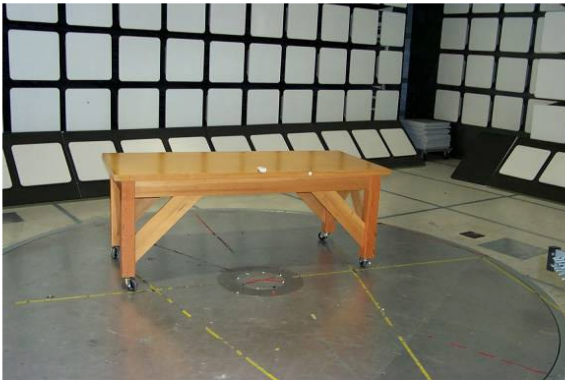
Figure 1 - Radiated Emissions Test Setup, Horizontal EUT Position
