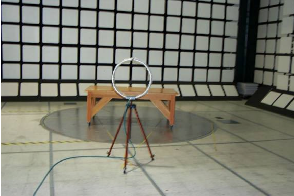
Figure 3 - Test setup, loop antenna at 3m test distance
