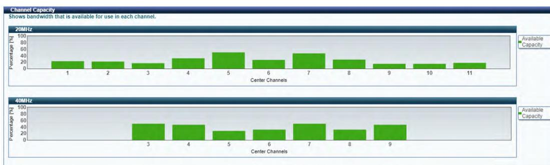
Shows interference level in each channel.
