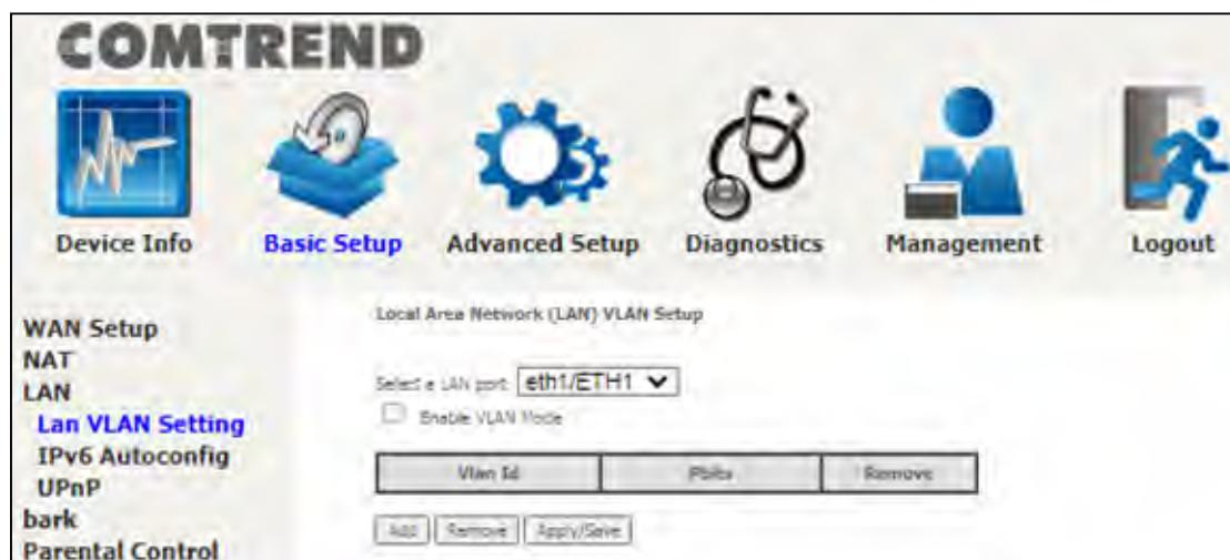
To enable VLAN Mode, check the checkbox and click the **Apply/Save** button.
