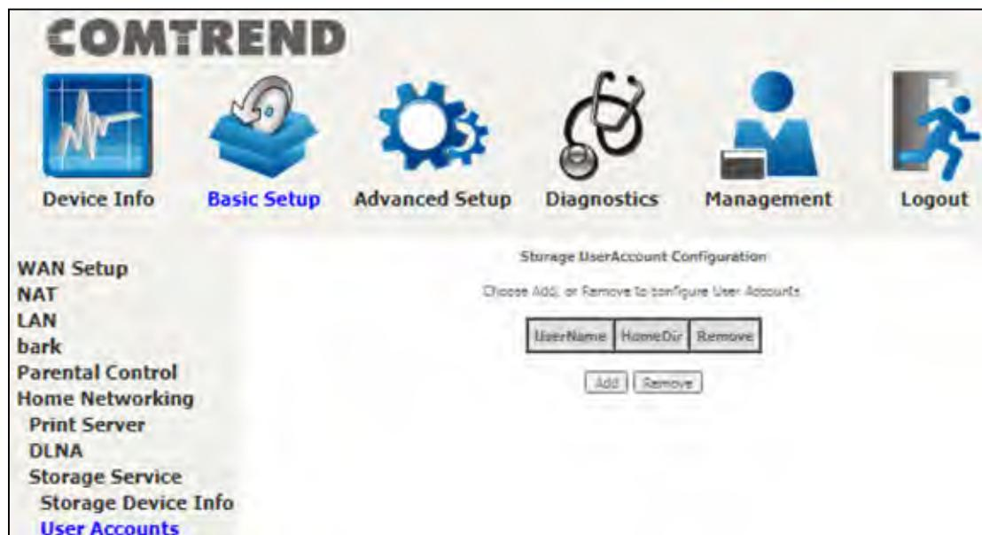
Click the **Add** button to display the following. volumeName would be disk1\_1 if only 1 USB has been plugged into the device.
