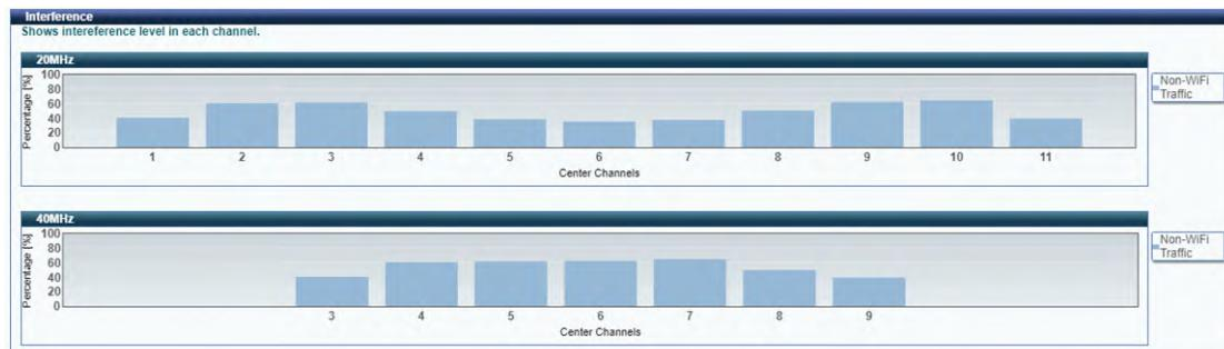
Shows the highest RSSI (Received Signal Strength Indicator) on each adjacent channel. Adjacent AP and associated stations are displayed for checking interference on those channels.
