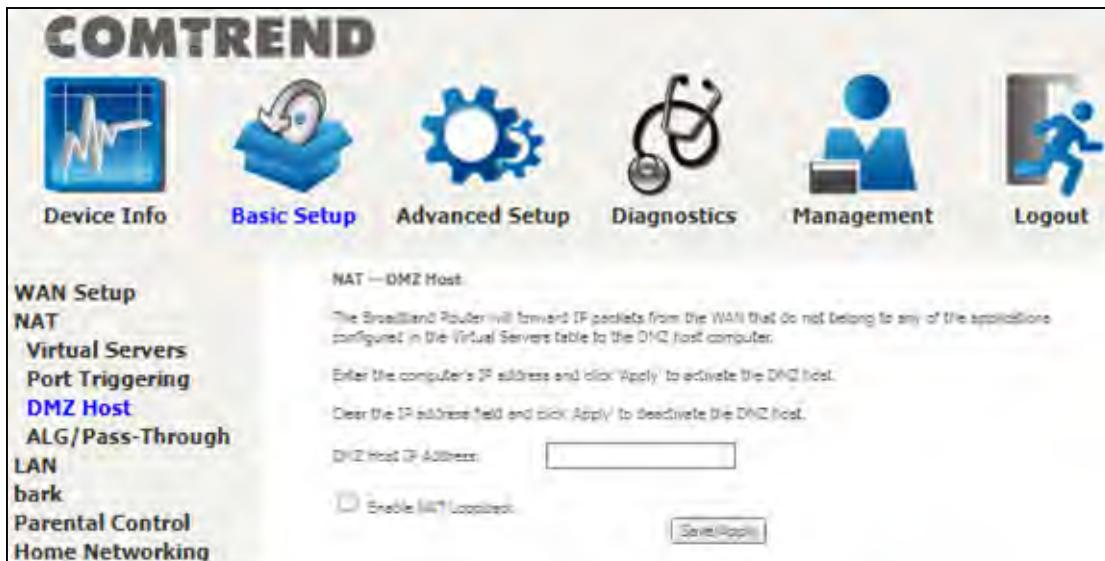
To **Activate** the DMZ host, enter the DMZ host IP address and click **Save/Apply**.
