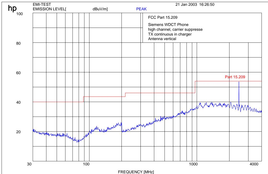
**f < 1 GHz : RBW/VBW: 100 kHz****f ≥ 1GHz : RBW/VBW: 1 MHz****Carrier was suppressed by a stubb tuner to avoid overload of the system.****LIMITS****SUBCLAUSE § 15.247 (c)**
