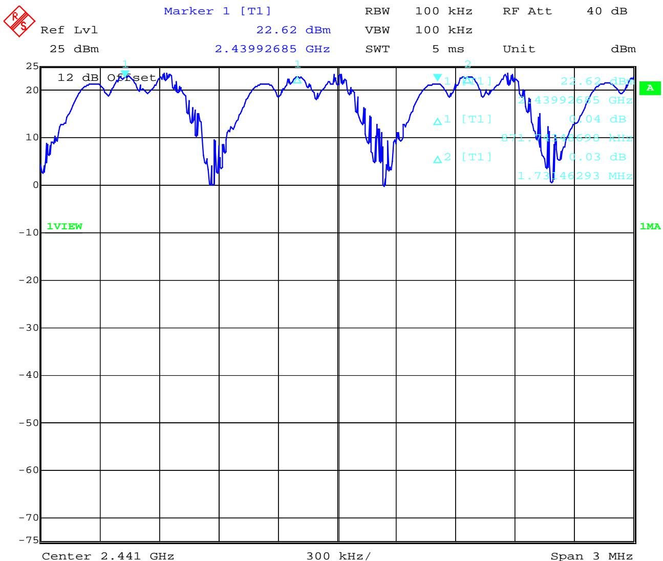
Limit: minimum 25 kHz or the 20 dB Bandwidth of the hopping system
