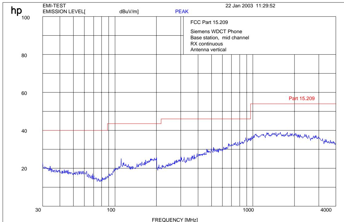
$f < 1 \text{ GHz}$  : RBW/VBW: 100 kHz $f \geq 1 \text{ GHz}$  : RBW/VBW: 1 MHz**Limits****SUBCLAUSE § 15.209**
