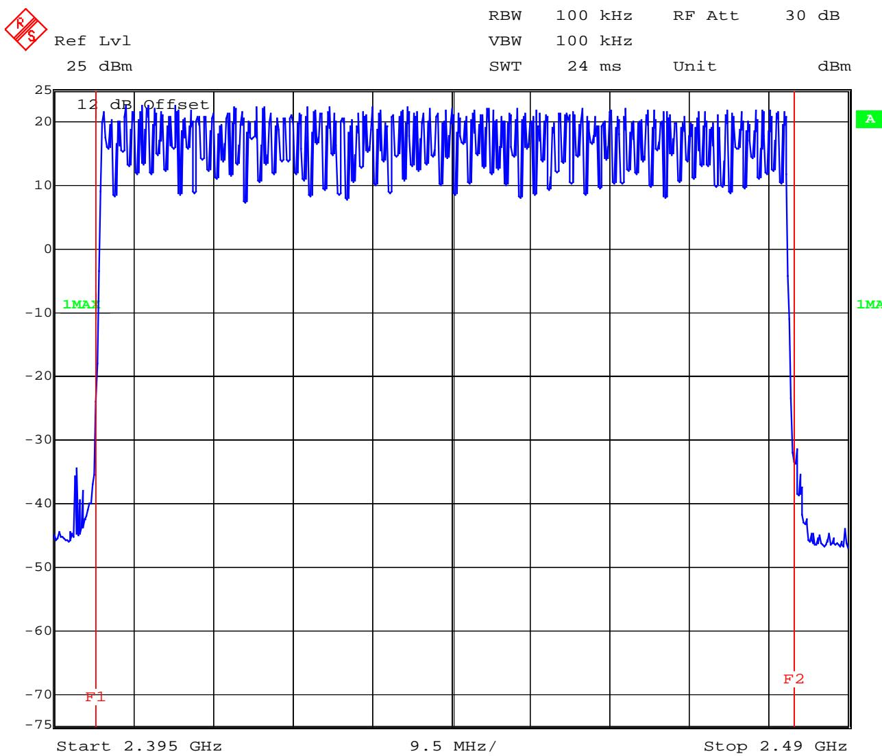
**Limit: at least 15 non-overlapping channels****REFERENCE NUMBER(S) OF TEST EQUIPMENT USED
