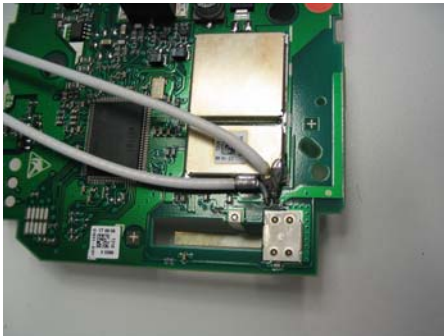
Figure 9: Antenna Measurement of BS
