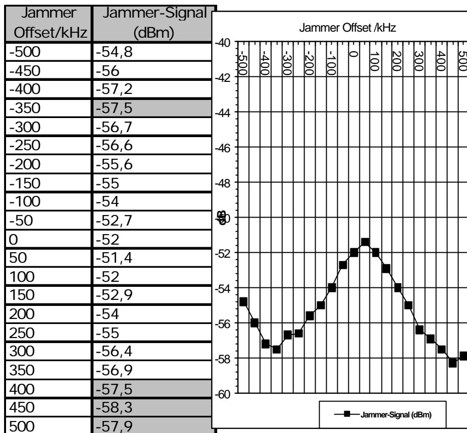
Disregarding the marked data points (-350, 400, 450, 500 kHz) the worst data point is at -400 kHz with a Jammer / Signal value of -11.8 dB.
