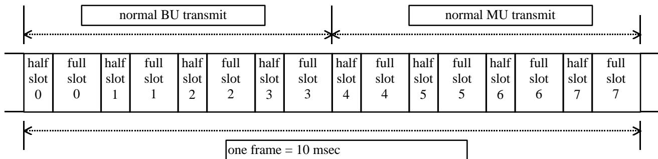
The half time slots are used for processor activities inside the system components and no transmissions (from either component) occur during these periods. Each full slot is equal to two half slots, which divides the total time for the period into 24 segments (half slot lengths).
