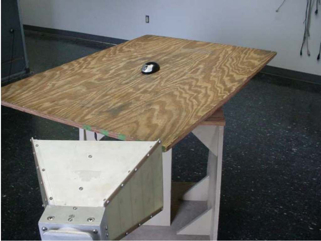
Microwave Radiated Emission Test Setup
