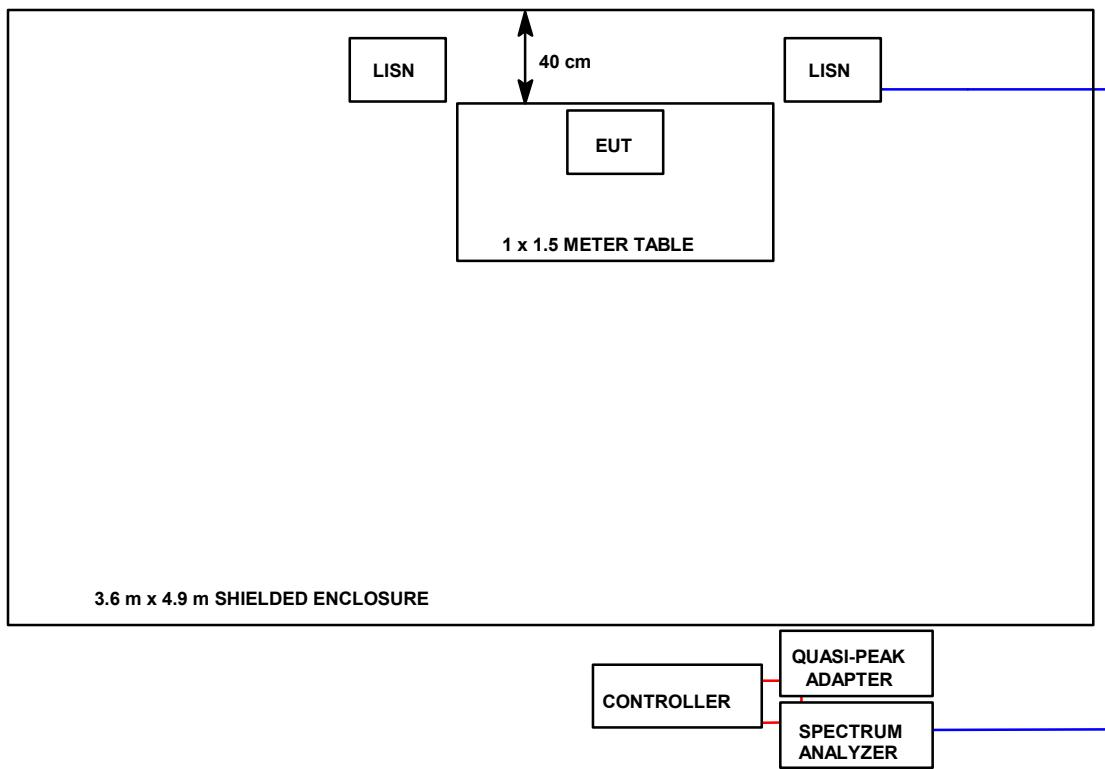
**FIGURE 2: Radiated Emissions Test Setup**
