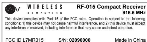
Stick the label in the inset on the back of the receiver. Replace the dummy serial number, **02090000**, with a real serial number.
