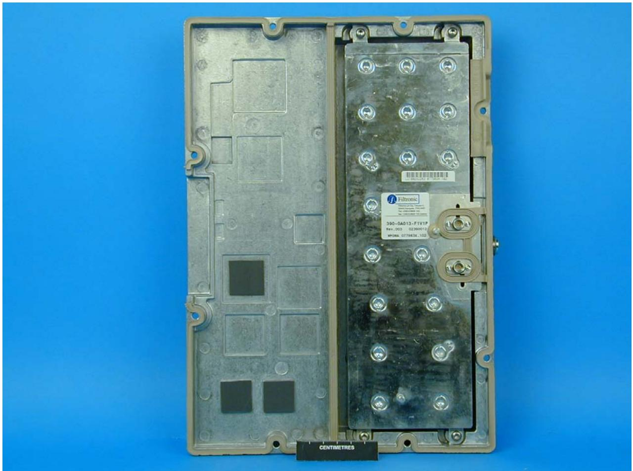
Photograph Number 4 – Internal – RF Filter Location
