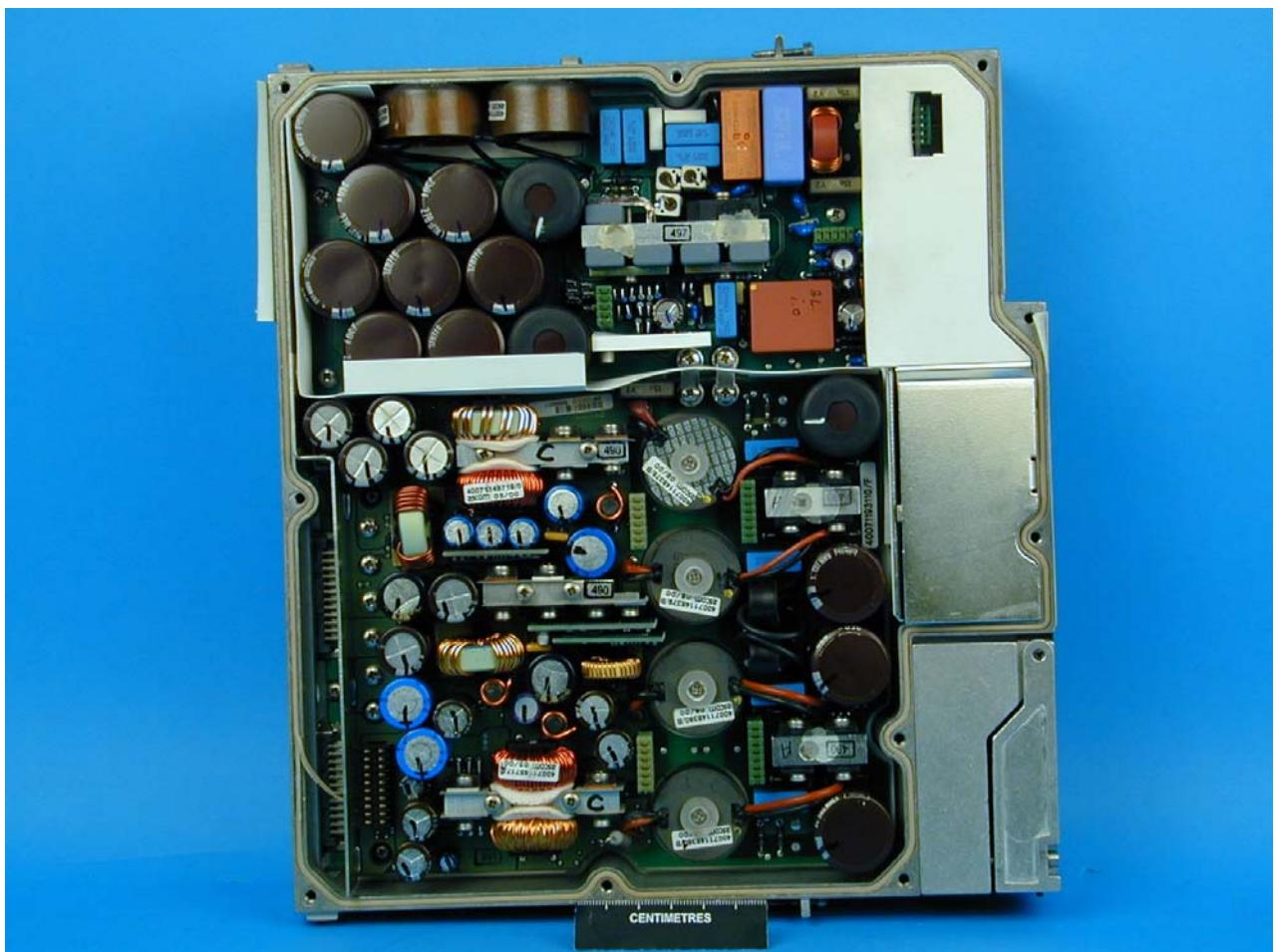
Photograph Number 35 – 110 AC PSU – Internal – Main PCB Circuitry
