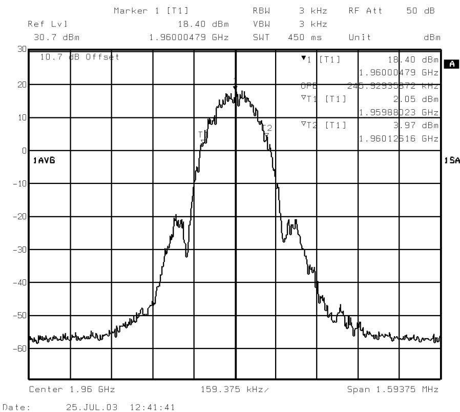
Measured Occupied Bandwidth = 245.929353kHz
