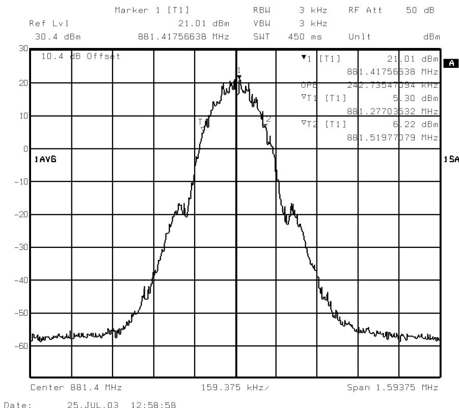
Measured Occupied Bandwidth = 242.735470kHz
