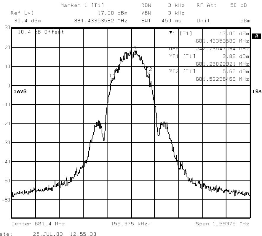
Measured Occupied Bandwidth = 242.735470kHz
