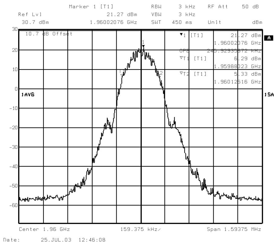
Measured Occupied Bandwidth = 245.929353kHz
