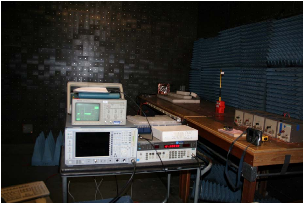
PHOTOGRAPH OF THE TEST SETUP FOR MEASUREMENTS OF MODULATION CHARACTERISTICS
