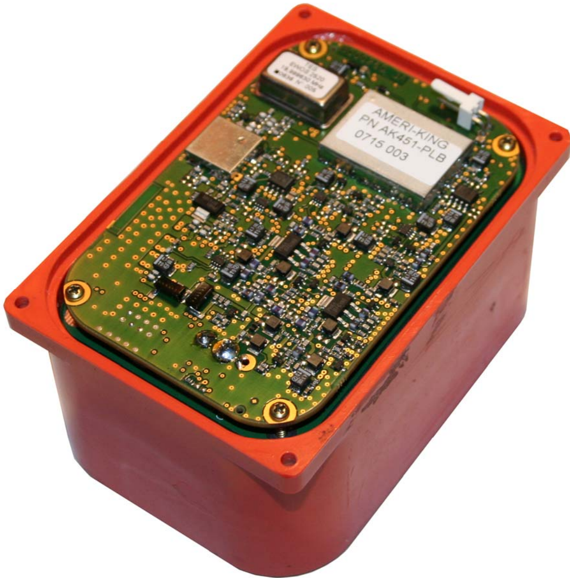
Beacon PCB assembly top side with case
