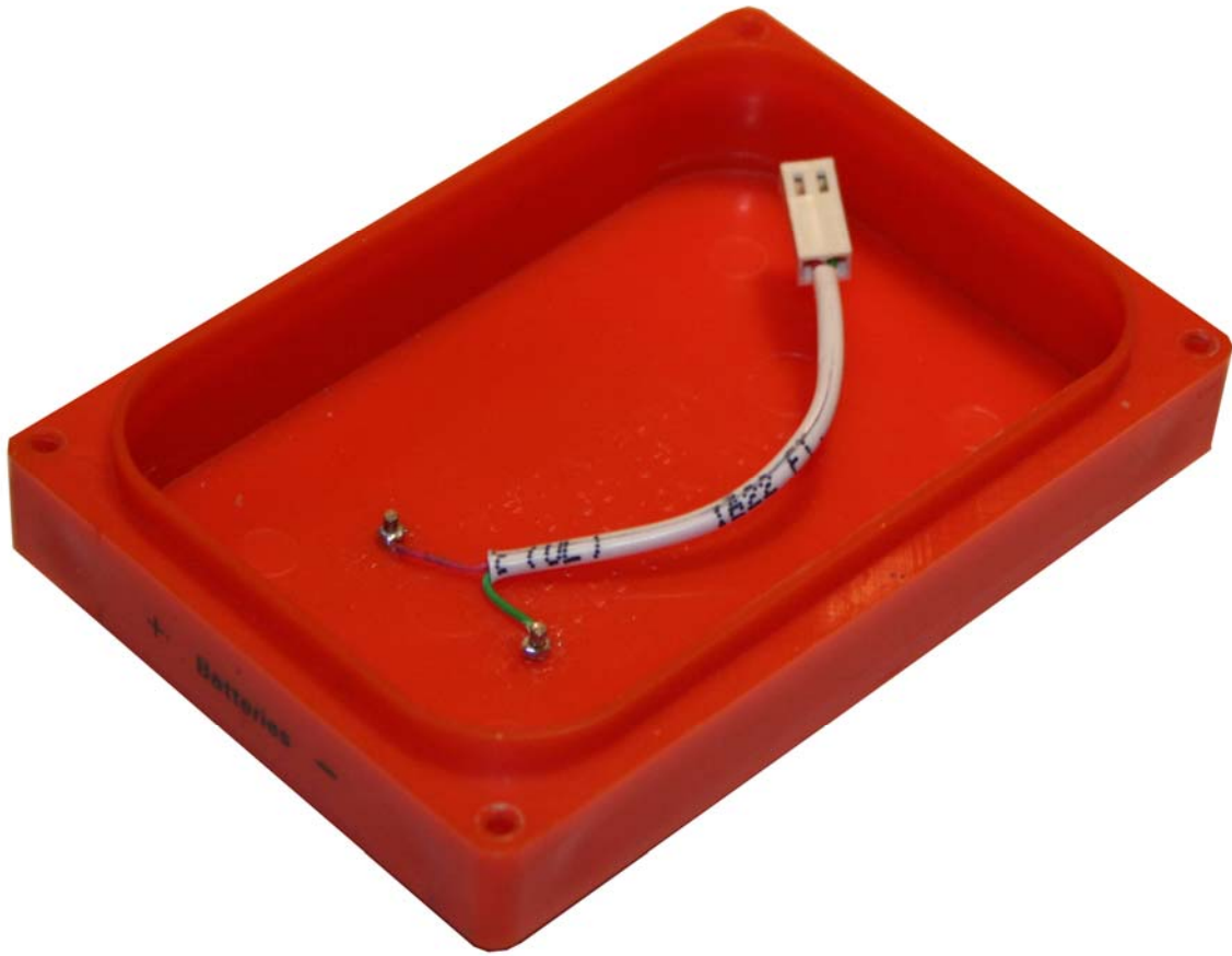
Battery assembly top side
