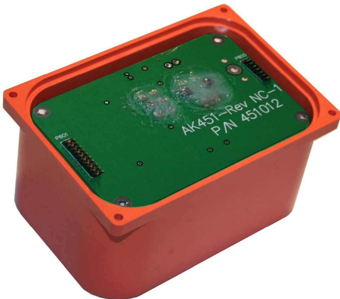
Switch PCB assembly top side with case
