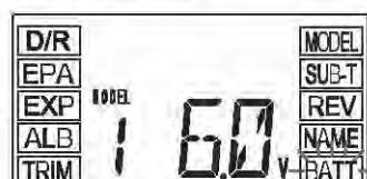
**!** The BATT menu is the transmitter's default menu. Each time the transmitter is turned ON, the BATT menu will be displayed. In addition, the BATT menu can be displayed at any time from within any other menu by pressing the MENU UP and MENU DOWN keys at the same time.
