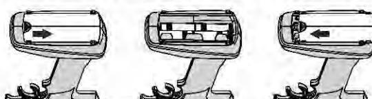
2) Install four fresh 'AA' Alkaline batteries into the battery holder, making sure that the polarity is correct. The direction that each battery should be installed is molded into the bottom of the battery holder (+ positive and - negative).
