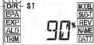
**⚠** Dual Rate is a percentage of End Point Adjustment. For example, if you set the Steering Dual Rate percentage value to 100%, the steering will travel the same amount as defined by your Steering End Point Adjustment programming. If you set the Steering Dual Rate percentage value to 50%, the steering will travel half that amount.
