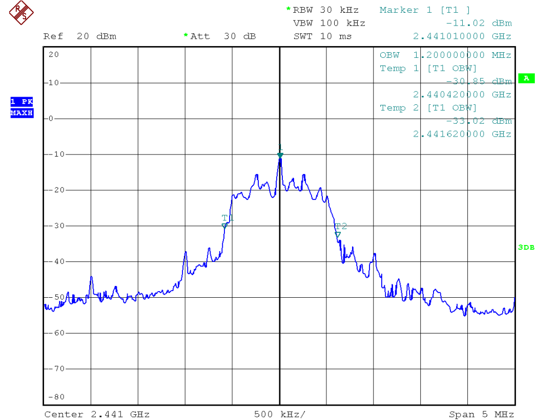
Figure 22- 99% Bandwidth Measurement (fc=2441MHz)
