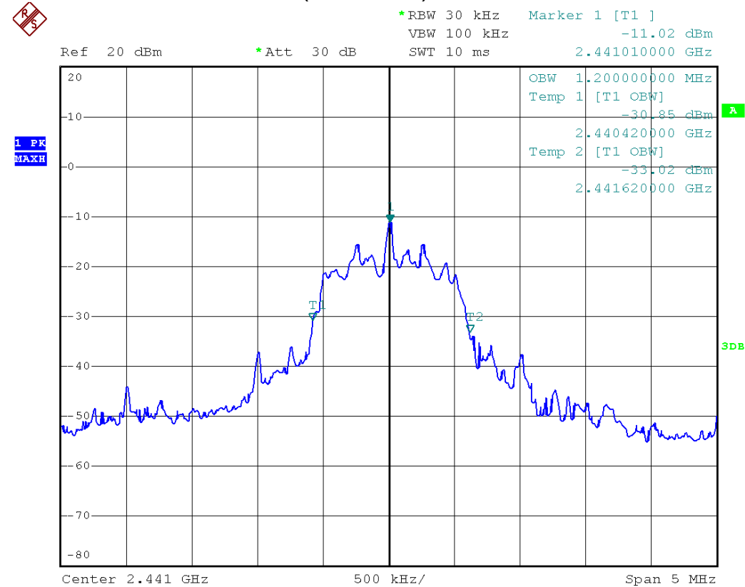
Figure 22- 99% Bandwidth Measurement (fc=2441MHz)
