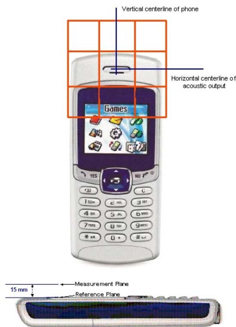
Figure 5.6-1: WD reference plane for RF emission measurement
