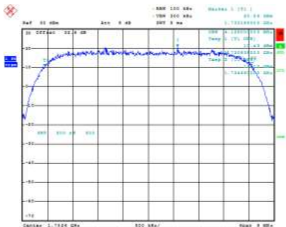
Figure 2-8b: Occupied Bandwidth, Band IV Middle Channel
