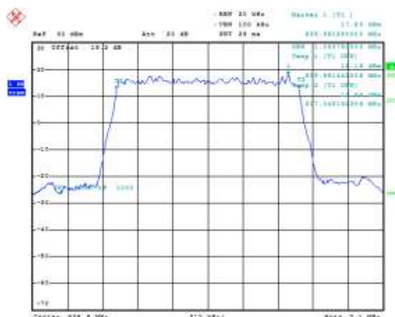
Figure 4-26a: Occupied Bandwidth, Band 5 Middle Channel, 1.4MHz BW, RB=6
