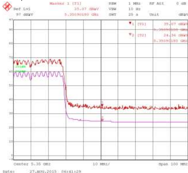
Figure 4-51: Band-Edge Compliance of RF Radiated Emission 802.11ac, MIMO, Ch. 62, 5310 MHz, Centre of Band-Edge: 5350 MHz
