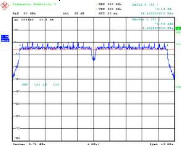
Figure 8-19: 6 dB Bandwidth Secondary, 802.11ac, Channel 140, MCS0 Mbps
