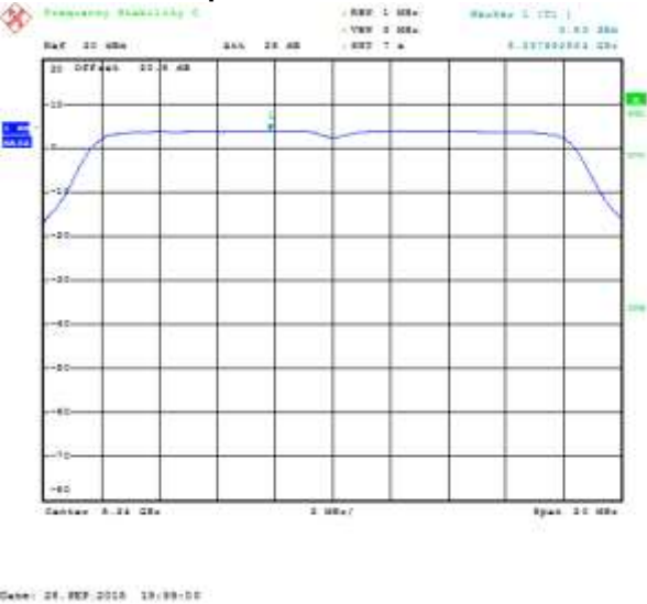
Figure 7-67: Peak Power Spectral Density SISO Primary, 802.11a, Channel 48, 6 Mbps
