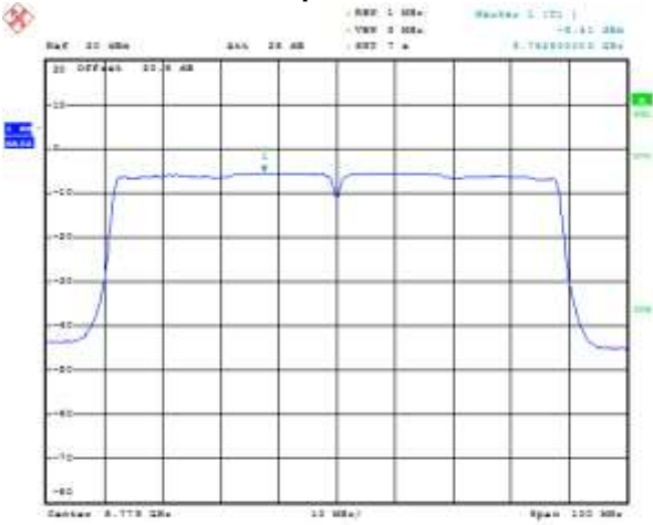
Figure 8-99: Peak Power Spectral Density SISO Primary, 802.11ac, Channel 155, MCS0 Mbps
