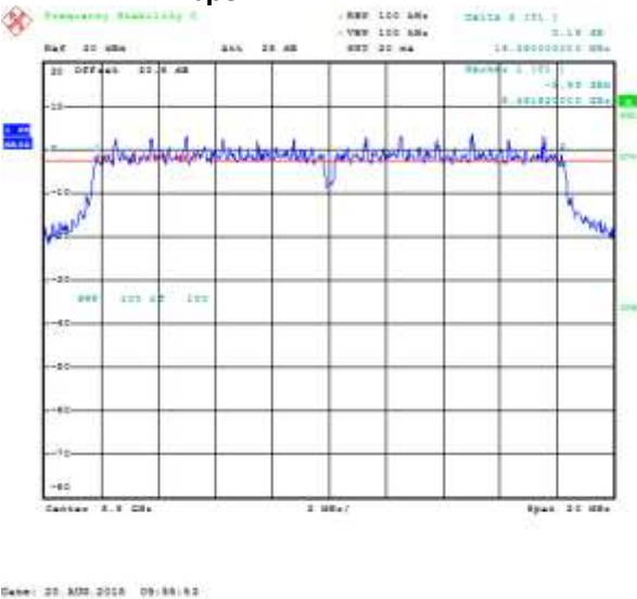
Figure 7-10: 6 dB Bandwidth Secondary, 802.11a, Channel 100, 6 Mbps
