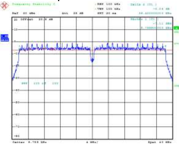
Figure 8-20: 6 dB Bandwidth Secondary, 802.11ac, Channel 149, MCS0 Mbps
