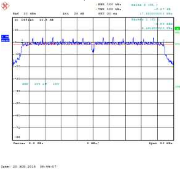
Figure 7-20: 6 dB Bandwidth Secondary, 802.11n, Channel 100, MCS 0
