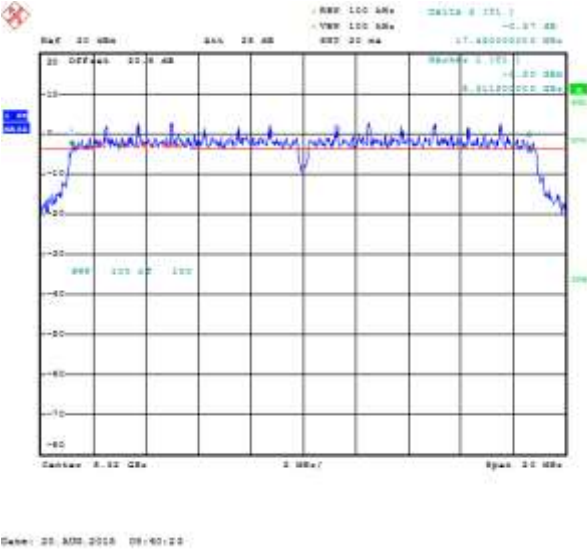
Figure 7-14: 6 dB Bandwidth Primary, 802.11n, Channel 64, MCS 0
