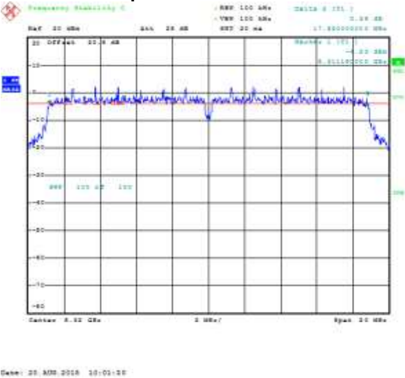
Figure 8-7: 6 dB Bandwidth Secondary, 802.11ac, Channel 64, 6 Mbps
