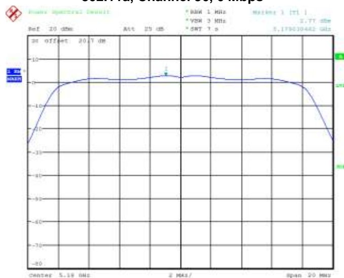
Figure 3-1: Peak Power Spectral Density 802.11a, Channel 36, 6 Mbps
