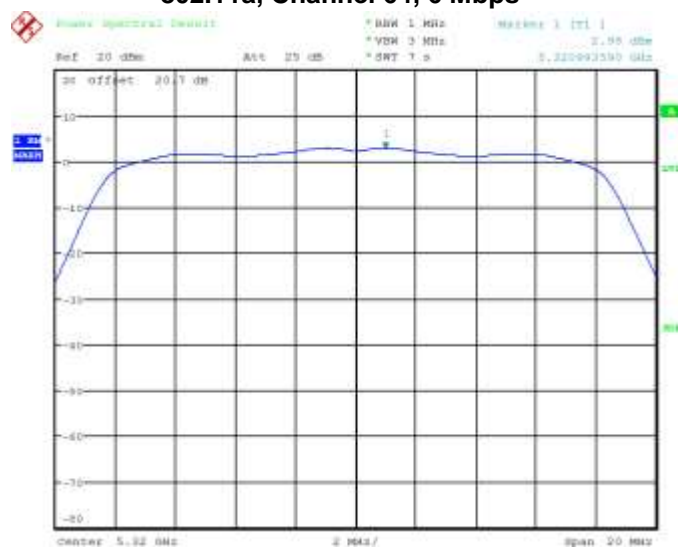
Figure 3-3: Peak Power Spectral Density 802.11a, Channel 64, 6 Mbps
