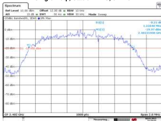
Figure 4-9: 20 dB Bandwidth Single freq., Static PBRs, 3-DH5
