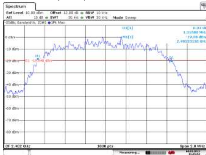
Figure 4-4: 20 dB Bandwidth Single freq., Static PBRS, 2-DH5
