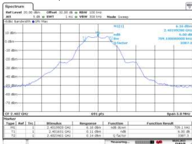
Figure 4-59: 6 dB Bandwidth LE, Channel 0
