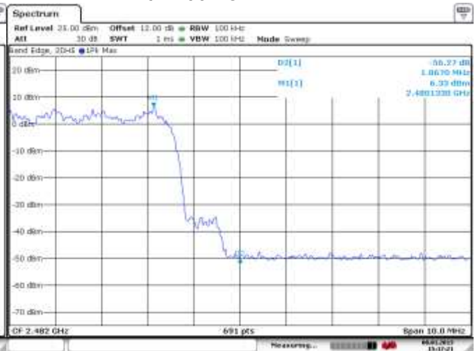
Figure 4-42: Band Edge Compliance Freq. Hopping, Static PBRS, 2-DH5
