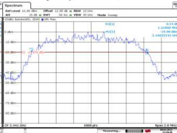
Figure 4-5: 20 dB Bandwidth Single freq., Static PBRS, 2-DH5
