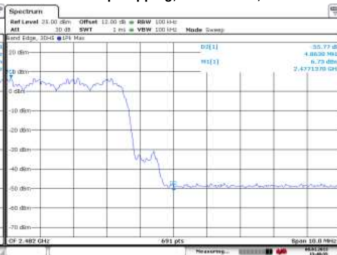
Figure 4-46: Band Edge Compliance Freq. Hopping, Static PBRS, 3-DH5
