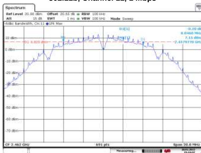
Figure 5-3: 6 dB Bandwidth 802.11b, Channel 11, 1 Mbps
