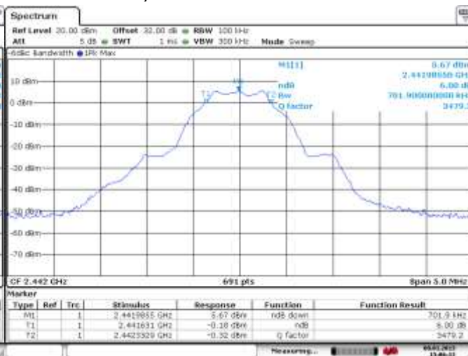
Figure 4-60: 6 dB Bandwidth LE, Channel 20
