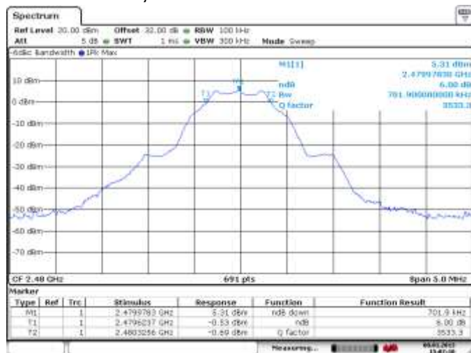
Figure 4-61: 6 dB Bandwidth LE, Channel 39
