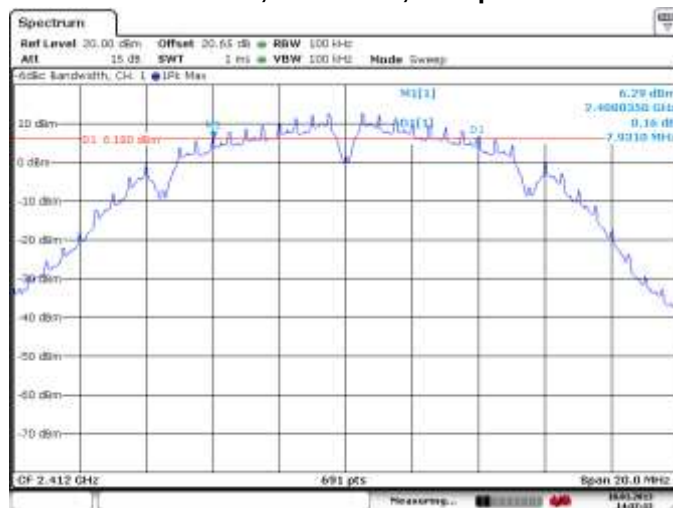
Figure 5-1: 6 dB Bandwidth 802.11b, Channel 1, 1 Mbps
