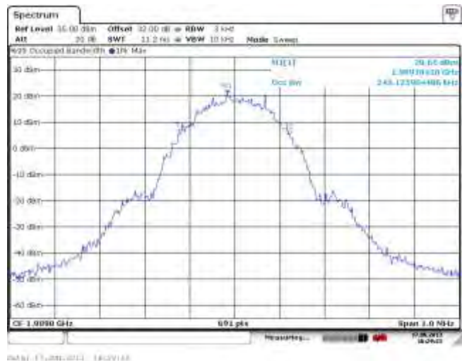
Figure 1-24a: Occupied Bandwidth, PCS1900 High Channel in GSM mode
