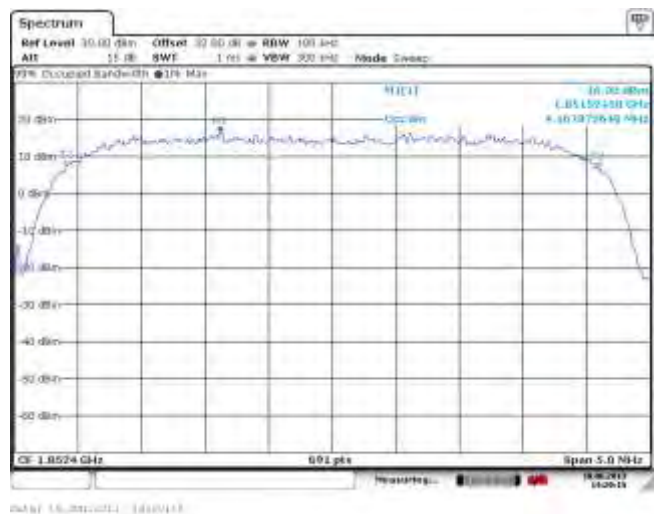
Figure 2-47a: Occupied Bandwidth, Band 2 HSUPA Low Channel
