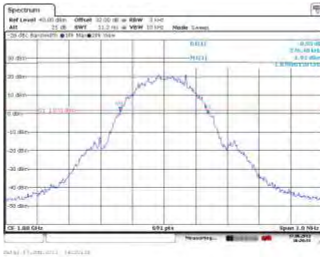
Figure 1-21a: -26dBc bandwidth, PCS1900 Middle Channel in GSM mode
