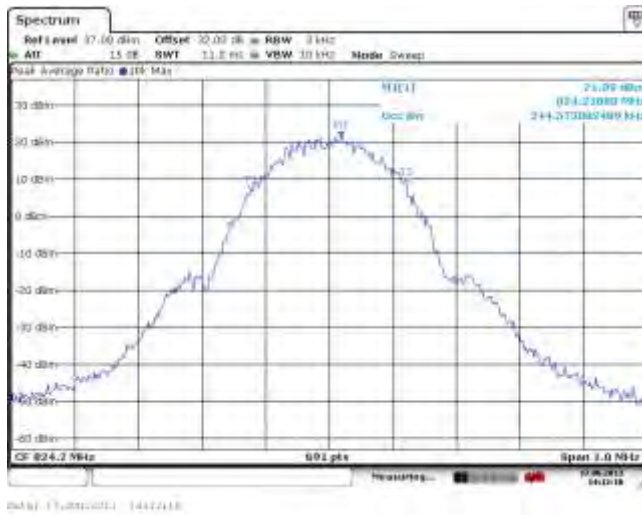
Figure 1-29a: Occupied Bandwidth, GSM850 Band, Low Channel in EDGE mode
