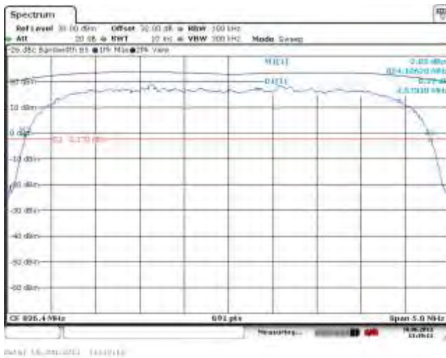
Figure 2-19a: -26 dBc Bandwidth, Band 5 Low Channel
