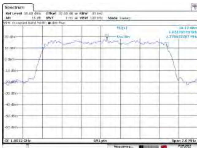
Figure 2-16a: Occupied Bandwidth PCS Loopback mode, Low Channel
