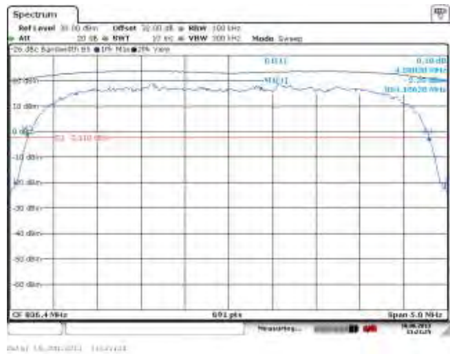
Figure 2-20a: -26 dBc Bandwidth, Band 5 Middle Channel
