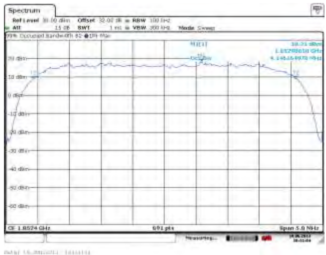
Figure 2-16a: Occupied Bandwidth, Band 2 Low Channel
