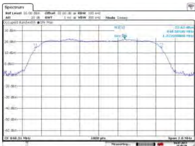
Figure 2-39a: Occupied Bandwidth Cellular EVDO mode, High Channel
