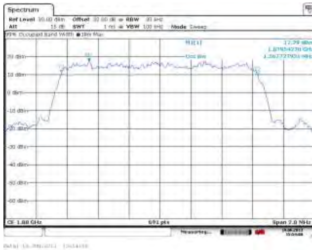
Figure 2-17a: Occupied Bandwidth PCS Loopback mode, Middle Channel
