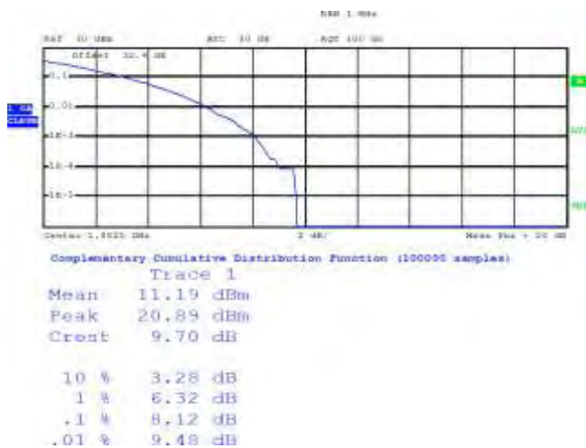
Figure 3-33a: Band 25, PAR, Mid Channel 10 MHz BW, RB = 25, QPSK
