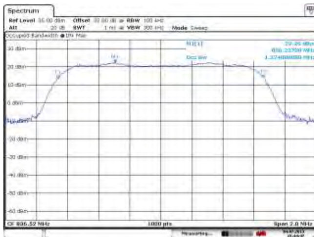
Figure 2-38a: Occupied Bandwidth Cellular EVDO mode, Middle Channel
