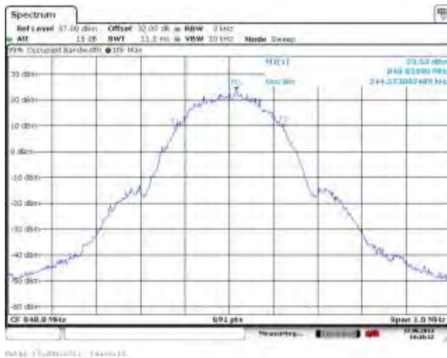
Figure 1-31a: Occupied Bandwidth, GSM850 band, High Channel in EDGE mode
