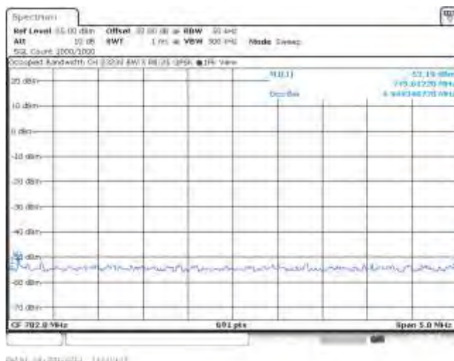
Figure 3-17a: Occupied Bandwidth, Band 5 Middle Channel, 5MHz BW, RB=25
