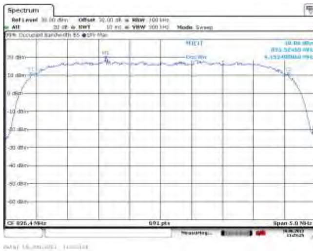
Figure 2-13a: Occupied Bandwidth, Band 5 Low Channel
