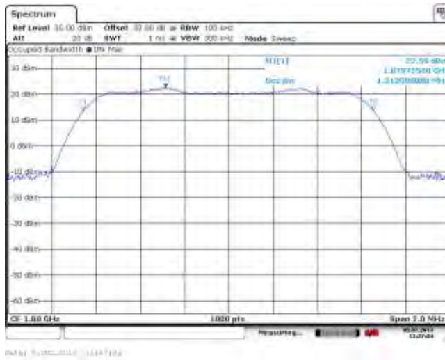
Figure 2-41a: Occupied Bandwidth PCS EVDO mode, Middle Channel
