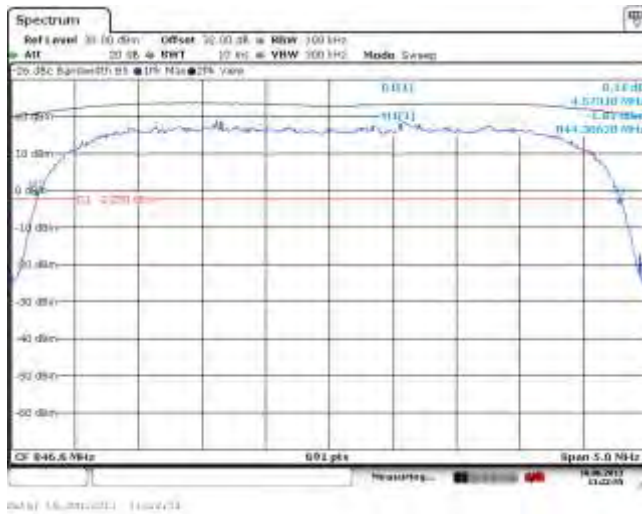
Figure 2-21a: -26 dBc Bandwidth, Band 5 High Channel
