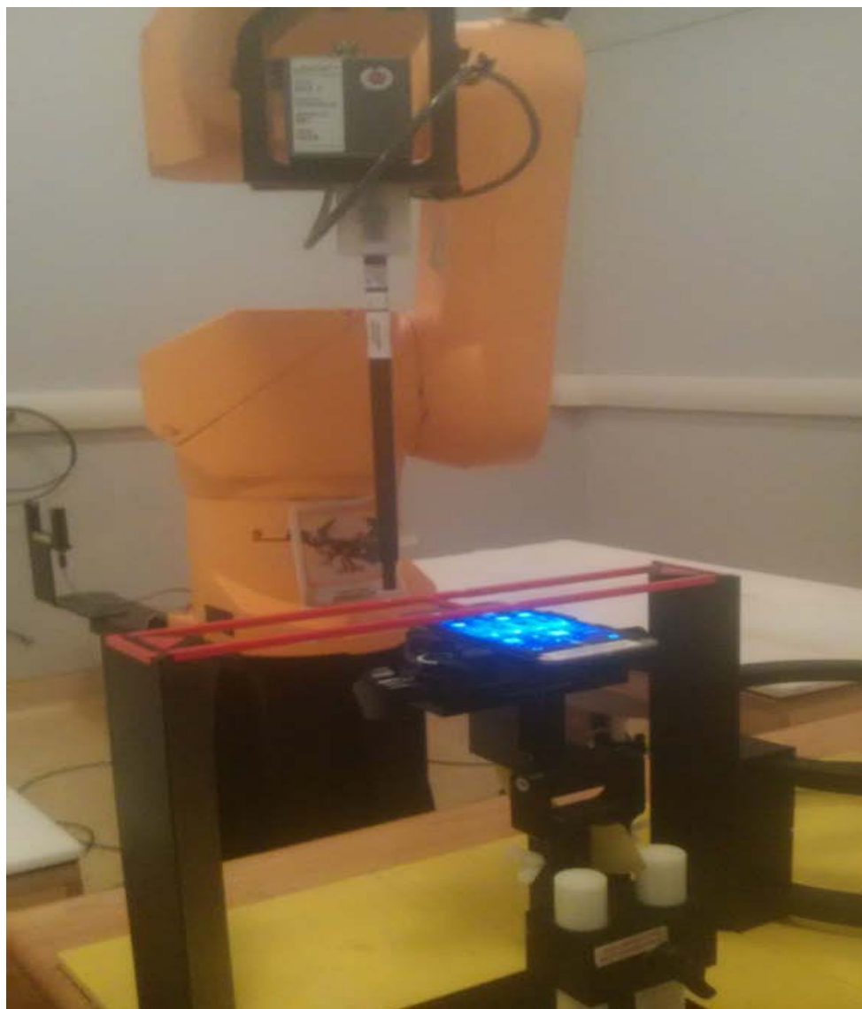
Figure C3 – HAC RF emission test setup
