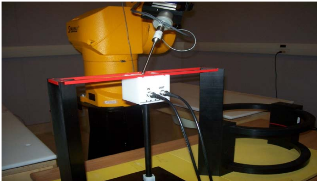
Figure E2: Ambient noise and system validation measurement setup
